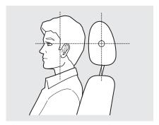
They are most effective when you adjust them so the center of the back of the occupant's head rests against the center of the restraint.
