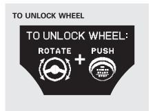
If the steering wheel is locked, the engine cannot start. The multi-information display shows you the above message and the indicator in the engine start/stop button blinks. To unlock the steering wheel, apply force by turning it left and right while pressing the engine start/stop button at the same time.
