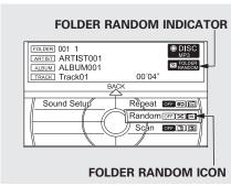
This feature, when activated, plays all files in the current folder in random order. To activate folder random play, push the interface selector down while playing a disc. Turn the interface dial to select Random on the AUDIO MENU, and press ENTER on the interface selector. Turn the interface dial to select the folder random icon, and press ENTER on the interface selector.
