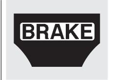
The audible alarm is a constant beeping sound; the visual alert is an amber colored BRAKE message that flashes on the multi-information display. If these alarms come on, take the appropriate means to prevent a collision (apply the brakes, change lanes, etc.).
