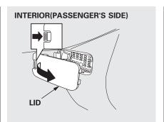
The passenger's side interior fuse box is on the lower passenger's side panel. To remove the fuse box lid, put your finger in the notch on the lid, and pull it upward slightly, then pull it toward you and take it out of its hinges.
