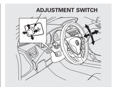
Move the steering wheel in, out, up, or down by pushing and holding the adjustment switch in that direction.
