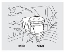
The fluid level should be between the MIN and MAX marks on the side of the reservoir. If the level is at or below the MIN mark, your brake system needs attention. Have the brake system inspected for leaks or worn brake pads. **Table of Contents**
