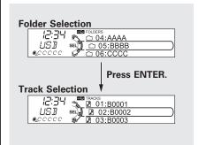
You can also select a folder or file from the list by using the selector knob. Push the selector knob (ENTER) to switch the display to the folder list, then turn the selector knob to select a folder. Press ENTER to change the display to the file list, then turn the same knob to select a file. Press ENTER to set your selection.
