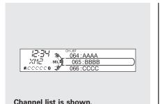
You can also select a channel or category from the list by using the selector knob. Push the selector knob (ENTER) to switch the display to the list displayed with three segments, then turn the knob to select a channel or category. Press the selector knob (ENTER) to set your selection or press the RETURN button to keep current selection.
