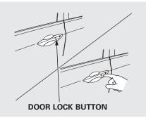
When you press the door lock button on the front door, all the doors and the tailgate will lock.
