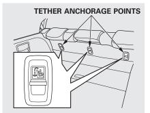
A child seat with a tether can be installed in any seating position in the back seat, using one of the anchorage points shown above.
