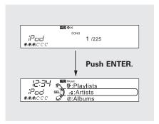
You can also select a file from any list on the iPod menu: playlists, artists, albums and songs, by using the selector knob. Push the selector knob (ENTER) to switch the display to an iPod menu, then turn the selector knob to select a desired list. Press ENTER to set your selection.
