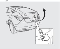
To open the tailgate, push up inside the handle, then lift up. To close the tailgate, use the inner handle to pull it down, then press down on the back edge.
