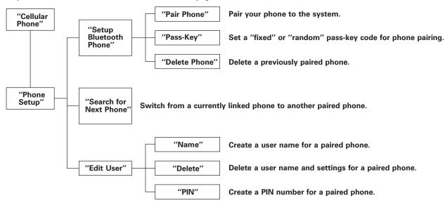
Voice commands can be used for all above options. Voice commands for the HFL system can only be used from the Cellular Phone screen. To quickly access the Cellular Phone screen, press the Pick-Up button on the steering wheel. Press and release the Talk button each time you give a command.
