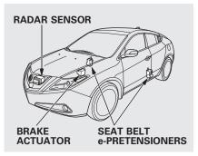
The CMBS consists of a radar sensor in the front grille, a brake actuator in the engine compartment, an indicator on the instrument panel, seat belt e-pretensioners on the front seats, and an on/off switch under the driver's side vent.
