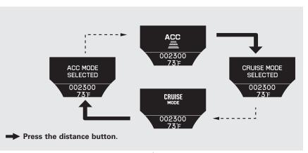
When you press the button, you will see CRUISE MODE SELECTED on the multi-information display for 2 seconds. To switch back to ACC, press and hold the distance button again for 1 second.
