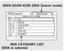
To activate RDS category search with the interface dial, push the AUDIO button to display the FM radio information on the screen. Push the interface selector down, and turn the interface dial to select RDS search. Press ENTER on the interface selector. The screen shows you the RDS category list.
