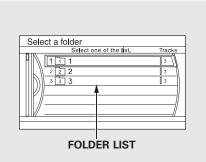
Using the interface selector, you can see the list of all the folders within a disc. While playing an MP3/WMA/AAC disc, push the interface selector up. The folder list in the currently playing disc will appear on the screen.
