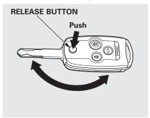
The master key can be retracted into the remote transmitter. To use the key, push the release button to release the key from the transmitter. The key should be fully extended. To retract the key, push the release button and at the same time push the key into the remote transmitter until it is securely latched.
