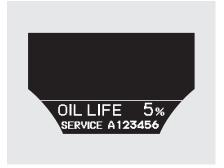
Press the SEL/RESET button on the steering wheel repeatedly to select the engine oil life. The message "SERVICE," along with "5%," and the maintenance item code are displayed on the multi-information display when the calculated engine oil life is 1 to 5 percent (see page 534).
