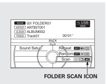
This function samples the first file in each folder within the USB flash memory device.
