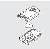
3. Replace the old battery with new battery. Place the battery so the + side is facing up. Snap the two halves of the remote case back together.
