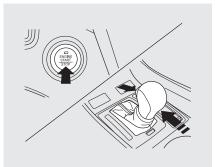
To turn the vehicle off when the vehicle is completely stopped, shift to Park (P), then press the engine start/stop button. The engine stops and the power mode switches from ON to VEHICLE OFF (LOCK).
