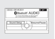
Press the AUDIO button to display the audio control display. Turn the dial to switch the setting between the resume/pause mode and the sound setup mode. Select Sound Setup, then press ENTER to set your selection.
