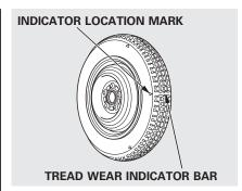
Replace the tire when you can see the tread wear indicator bars. The replacement should be the same size and design tire, mounted on the same wheel. The spare tire is not designed to be mounted on a regular wheel, and the spare wheel is not designed for mounting a regular tire. If you have a flat tire while driving, stop in a safe place to change it. Drive slowly along the shoulder until you get to an exit or an area to stop that is far away from the traffic lanes.
