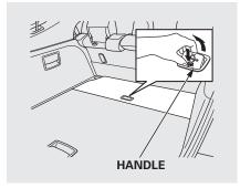
4. Push the rear edge of the handle to raise the handle and pull up the handle to raise the front cargo area floor.
