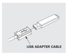
2. Connect the USB flash memory device to the USB adapter cable correctly and securely.
