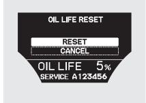
4. Select "RESET" by pressing the INFO (▲/▼) button, then press the SEL/ RESET button to reset the engine oil life display. The maintenance item code (s) will disappear, and the engine oil life will reset to "100." If you want to cancel the oil life reset mode, select "CANCEL."
