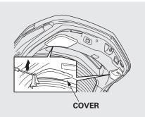
1. Open the tailgate. Place a cloth on the edge of the light assembly cover to prevent scratches. Remove the cover by carefully prying in the notch on its middle edge with a flat-tip screwdriver.
