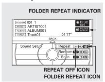
This feature, when activated, replays all files on the selected folder in the order they are compressed. To activate folder repeat play, push the interface selector down while playing a disc. Turn the interface dial to select Repeat on the AUDIO MENU, and press ENTER on the interface selector. Turn the interface dial to select the folder repeat icon, and press ENTER on the interface selector.
