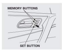
3. Press and release the SET button on the door. You will hear a beep. Immediately press and hold one of the memory buttons (1 or 2) until you hear two beeps. The indicator in the memory button will come on. The current positions of the driver's seat, steering wheel, and outside mirrors are now stored.
