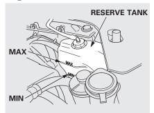
Look at the coolant level in the radiator reserve tank. Make sure it is between the MAX and MIN lines. If it is below the MIN line, see **Adding Engine Coolant** on page 548 for information on adding the proper coolant.
