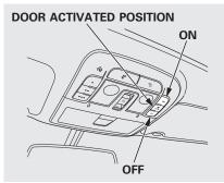
Your vehicle has the light control buttons on the front ceiling. With these buttons, you can select three positions: OFF, DOOR (door activated position), and ON.
