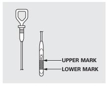
Remove the dipstick again, and check the level. It should be between the upper and lower marks.
