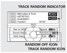
This feature plays the tracks within a disc in random order. When playing MP3, WMA or AAC format discs, all the tracks within the disc are played in random order, regardless of the configuration of the folder.
