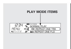
To cancel the selected mode, press the SETUP button and turn the selector knob to show "PLAY MODE," then press ENTER. When you see "NORMAL PLAY," press ENTER again. **REPEAT ONE TRK** – This feature continuously plays a file. Select "NORMAL PLAY" to turn it off. Pressing either side of the SKIP bar also turns off this feature.
