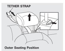
1. After properly securing the child seat (see page 51), lift the head restraint, then route the tether strap over the seat-back and through the head restraint legs.
