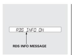
To switch the RDS INFO display function on and off, press and release the TITLE side of the SCAN/TITLE bar. With the system on, you will see the "RDS INFO ON" message on the display. If the station you are listening to is an RDS station, the displayed frequency switches to the station name.
