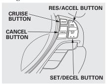
1. Push in the CRUISE button MAIN button (models with adaptive cruise control) on the steering wheel. The CRUISE MAIN indicator on green ACC indicator (models with ACC) on the instrument panel comes on.
