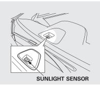
The climate control system has two sensors: a sunlight sensor on top of the dashboard, and a temperature and humidity sensor next to the steering column. Do not cover the sensors or spill any liquid on them.
