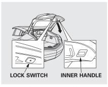
To close the tailgate, use the inner handle to pull it down, then press down on the back edge.
