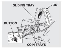
Your vehicle has a multi-function center console. It includes beverage holders, storage compartments, an armrest, storage trays for coins or small items, and a sliding tray.
