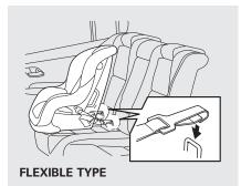
Other LATCH-compatible seats have a flexible-type connector as shown above.
