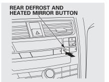
The outside mirrors are heated to remove fog and frost. With the ignition switch in the ON (II) position, turn on the heaters by pressing the button. The indicator in the button comes on as a reminder. Press the button again to turn the heaters off. Pressing this button also turns the rear window defogger on and off.
