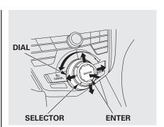
The dial turns left and right. Use it to make selections or adjustments to a list or menu on the screen.
