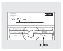
TUNE — Use the TUNE bar to tune the radio to a desired frequency. Press the ▶ side of the bar to tune to a higher frequency, or the ◀ side to tune to a lower frequency. To tune with the interface dial, push the interface selector down, and turn the interface dial to select Tune. Then press ENTER on the interface selector, and turn the interface dial to the desired frequency. To exit the TUNE mode, press ENTER on the interface selector, then push the interface selector up to go back.
