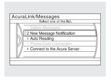
To access the following functions, press the INFO/PHONE button, then bring up the INFO screen. Select Setup with the interface selector to view the SETUP screen. Push the interface selector to the right to select Other, then rotate the interface knob to select AcuraLink/Messages.
