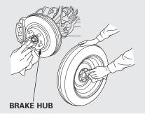
13. Before mounting the spare tire, wipe any dirt off the mounting surface of the wheel and hub with a clean cloth. Wipe the hub carefully; it may be hot from driving.
