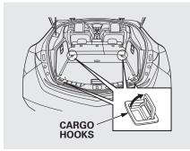
To secure cargo, use the four floor hooks in the cargo area. Make sure all stored items are secured before driving. The cargo area carpets are loop-type construction. If snags occur from sharp or rough objects, do not pull the loose threads to remove them. Cut all loose threads with a scissors to prevent carpet runs.
