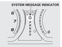
If there is a problem with your vehicle, for example, the engine oil level is low or a door is not fully closed, the multi-information display will show you the problem. It does this by interrupting the current display with one or more messages.
