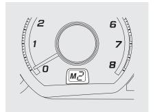
Using a paddle shift mode, the gear position indicator shows you the selected gear number (see page 482).
