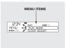
You can select any type of repeat and shuffle mode by using the SETUP button and the selector knob. Press the SETUP button to display the menu items, then turn the selector knob to select "PLAY MODE." Press ENTER to set the selection.
