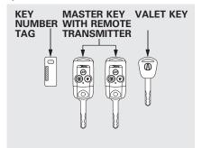
The master key fits all the locks on your vehicle. The valet key works only in the ignition and the driver's door lock. You can keep the glove box locked when you leave your vehicle and the valet key at a parking facility.
