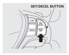
3. Press and release the SET/ DECEL button on the steering wheel, then release the accelerator pedal.
