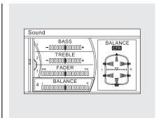
You can also adjust the sound by pushing the J/J (Sound) button repeatedly. Each mode is shown in the display as you push the button.
