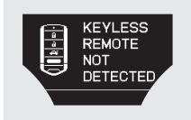
If you take the keyless access remote out of the vehicle and close the door with the power mode ON, the inside and outside beepers sound and a "KEYLESS REMOTE NOT DETECTED" message will be displayed on the multi-information display.
