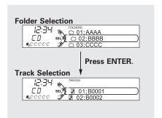
In MP3 or WMA mode, you can also select a folder or track/file from the list by using the selector knob. Push the selector knob (ENTER) to switch the display to the list displayed with three segments, then turn the knob to select a folder. Press the selector knob (ENTER) to change the display to the track/file list, then turn the same knob to select a track/file. Press the selector knob (ENTER) to set your selection.
