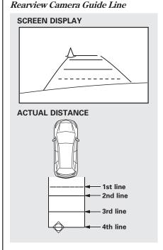
The camera display has parking guide lines that indicate distance from your vehicle.
