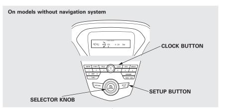
On models without navigation system To adjust the clock setting:
