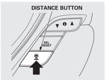
To switch from ACC to cruise control, press the distance button on the steering wheel, and hold it for 1 second.
