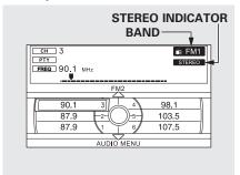
The power mode must be in ACCESSORY or ON. Press the AUDIO button to view the audio control display. Turn the system on by pressing the VOL/ & knob or the AM/FM button. Adjust the volume by turning the VOL/ & knob.
