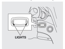
Your vehicle has a keyless access remote slot light. The light comes on when you:
