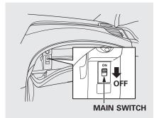
This switch is in the glove box. You can cancel the keyless access system features, which are locking/unlocking the doors, unlocking the tailgate, and starting the engine while carrying the keyless access remote. To cancel the system, turn the keyless access system main switch off by pushing it down.
