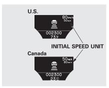
If you change the speed unit measurement from the factory default setting, the initial speed unit measurement is shown under the current unit.
