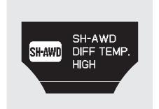
If the SH-AWD indicator blinks while driving, it indicates the differential temperature is too high. You will also see an "SH-AWD DIFF TEMP. HIGH" message on the multi-information display. If this happens, pull to the side of the road when it is safe, shift to Park, and let the engine idle until the indicator goes out. If the indicator does not go out, take your vehicle to a dealer to have it checked.
