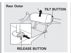
If for some reason you need to remove the rear outer head restraint, push the tilt button, then fold the head restraint backward. Push the release button, then pull the restraint out of the seat-back.
