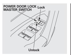
To lock all doors and the tailgate, press the front of the master door lock switch on either front door, pull the lock tab rearward on the driver's door, or use the key on the outside lock on the driver's door
