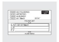
You can also select a folder or file from the list by using the interface dial. Press the AUDIO button to show the audio display on the navigation screen. Use the interface dial to highlight the file, then press ENTER to set your selection.
