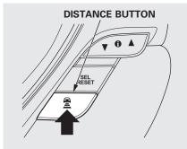
With ACC on, the distance between your vehicle and the vehicle ahead of you is controlled and maintained. You can change this distance to one of three ranges: long, middle, or short.
