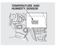
The humidity sensor helps reduce window fogging and also monitors and adjusts cabin humidity by automatically changing the mode to defrost.
