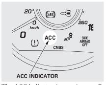
The ACC indicator (orange) normally comes on for a few seconds when you select the ON mode by operating the engine start/stop button (see page 194). If it comes on at any other time, there is a problem in the ACC system. If this happens, take the vehicle to your dealer to have it checked.
