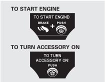
After you unlock and open the driver's door, you will see the "TO START ENGINE:" message on the multi-information display. The "TO TURN ACCESSORY ON:" message will be shown after three seconds. The display switches between the "TO START ENGINE:" and "TO TURN ACCESSORY ON:" messages every three seconds.
