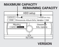
You can check the HDD Audio capacity and remaining space as well as the Gracenote Music Recognition Service (CDDB) version included with the navigation system on the HDD Setup screen.
