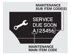
When the remaining engine oil life is 15 to 6 percent, the multi-information display shows a "SERVICE DUE SOON" message along with the maintenance item code(s) indicating the main and sub items required at the time of the oil change. Refer to page 542 for a complete list of the maintenance main items and sub items.
