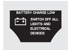
IGN ACCESSORY (I) or LOCK (0) – Follow the multi-information display message and turn off all electrical devices. Driving the vehicle will recharge the battery, however the vehicle may not start. If no start, see jump starting (page 587), or contact your dealer.
