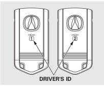
When you unlock the door with your remote, each remote activates the keyless memory settings related to that remote. The driver's ID (Driver 1 or Driver 2) is shown on the back of each remote.
