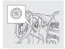
The ignition switch has four positions: LOCK (0), ACCESSORY (I), ON (II), and START (III).
