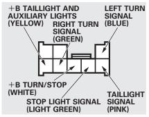
Your vehicle has a trailer lighting connector located under the right side tool case in the cargo area. Refer to the drawing above for the wiring color code and purpose of each pin.
