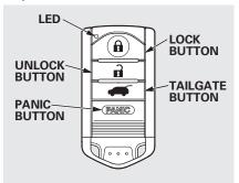
LOCK – Press this button once to lock all doors and the tailgate. Some exterior lights will flash. When you push the LOCK button twice within 5 seconds, you will hear a beep to verify that the doors and the tailgate are locked and the security system is set.
