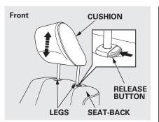
Adjusting the Head Restraint
