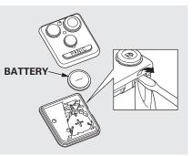
3. Place a cloth on the edge of the keypad to prevent scratches, and remove the upper half by carefully prying on the edge with a small flat-tip screwdriver.
