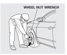
9. Loosen each wheel nut 1/2 turn with the wheel nut wrench.
