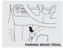
To apply the parking brake, push the pedal down with your foot. To release it, push on the pedal again. The parking brake indicator on the instrument panel should go out when the parking brake is fully released (see page 66).
