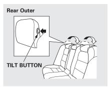
To lower either rear outer head restraint for better visibility, press the tilt button on the side of the head restraint. It folds down backward. To raise the rear outer head restraint, pull it up from the rear by hand. Make sure the head restraint locks in position when you lower or raise it.
