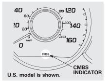
This indicator comes on for several seconds when you select the ON mode by operating the engine start/stop button (see page 194). It also comes on and stays on when you turn the CMBS off by pressing the CMBS OFF button.
