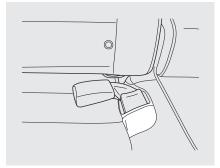
1. Store the center seat belt buckle into the pocket in the rear seat-back.
