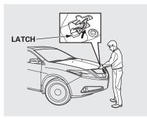
2. Put your fingers under the front edge of the hood near the center. Slide your hand to your left until you feel the hood latch handle. Push this handle up until it releases the hood. Lift up the hood.
