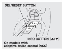
With the ignition switch in the ON (II) position, the multi-information display changes as shown on page 81 each time you press the INFO (▲/▼) button or the SEL/RESET button.
