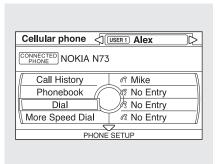
During a call, HFL allows you to talk up to 30 minutes after you remove the key from the ignition switch. However, this may weaken the vehicle's battery.
