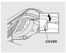
Open the tailgate. Place a cloth on the edge of the light assembly cover to prevent scratches.
