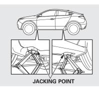
10. Place the jack under the jacking point nearest the tire you need to change. Turn the end bracket clockwise until the top of the jack contacts the jacking point. Make sure the jacking point tab is resting in the jack notch.
