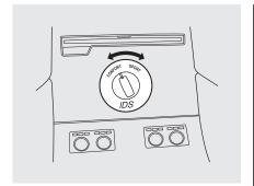
Turn the Integrated Dynamics System (IDS) switch located on the center console to select the comfort and sport mode.
