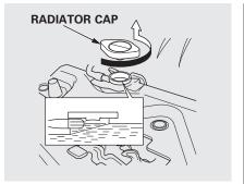
3. Remove the radiator cap by pushing down and turning counterclockwise.
