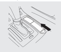
Your vehicle has two accessory power sockets. One is next to the shift lever. The other is in the console compartment.
