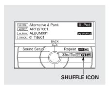
**SHUFFLE** – This feature shuffles playback of tracks contained within the iPod. This function can be established at the same time that Repeat Playback is set up.
