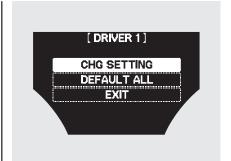
When you want to change the vehicle control settings, press the INFO (▲/▼) button to select CHG SETTING, then press the SEL/RESET button.
