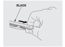
3. Remove the blade from its holder by grabbing the tabbed end of the blade. Pull firmly until the tabs come out of the holder.
