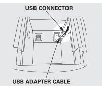
1. Unclip the USB connector by pulling it up, and pull out the USB adapter cable in the console compartment.
