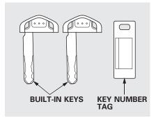
Each keyless access remote has the built-in key. This key is used to lock/unlock the doors when the remote battery becomes weak and the power door lock/unlock operation is disabled. You cannot start the engine with this key.
