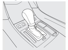
To shift from Park to any position, press firmly on the brake pedal, and press the release button on the front of the shift lever, then move the lever. You cannot shift out of Park when the ignition switch is in the LOCK (0) or ACCESSORY (I) position.
