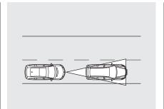
When a vehicle ahead is within ACC range and going at a steady speed Your vehicle follows the vehicle ahead of it, keeping a constant distance. ACC will not keep your vehicle at a constant distance if the vehicle ahead of you goes out of range of your set speed.
