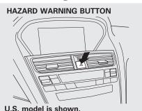
Push the button between the center vents to turn on the hazard warning lights (four-way flashers). This causes all four outside turn signals and both indicators in the instrument panel to flash. Use the hazard warning lights if you need to park in a dangerous area near heavy traffic, or if your vehicle is disabled.
