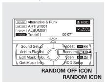
This function plays the tracks on the HDD in random order. To activate random play, push the interface selector down during track playback. Turn the interface dial to select Random on the HDD AUDIO MENU. Press ENTER on the interface selector.
