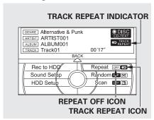
To replay the current track continuously, push the interface selector down while playing a disc. Turn the interface dial to select Repeat on the AUDIO MENU, and press ENTER on the interface selector. Turn the interface dial to select Repeat icon, and press ENTER on the interface selector.
