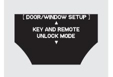
To select whether the driver's door unlocks or all the doors unlock when you unlock the doors with the remote transmitter/keyless access remote, follow these instructions.
