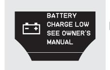
IGN ON (II) – Immediately turn off all electrical devices (interior lights, air conditioning, audio, heated seats, etc.). Try not to operate other electrically operated controls such as the power windows. Driving the vehicle will recharge the battery. If the message continues to display while driving, see your dealer.
