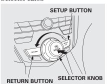
Most audio system functions can be controlled by standard buttons, bars, and knobs. In addition, you can access some functions by using the selector knob on the audio system.
