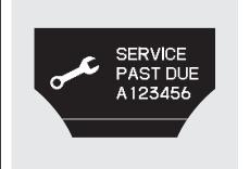
If the indicated maintenance service is not done and the remaining engine oil life reaches 0%, the multi-information display will show the message "SERVICE PAST DUE" and the maintenance item code(s). This message is displayed when the total distance traveled is less than 10 miles (for U.S. models) or 10 km (for Canadian models) after the engine oil life became 0%.
