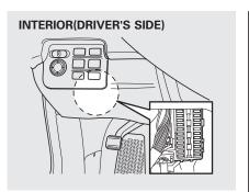
The vehicle's fuses are located in four fuse boxes.
