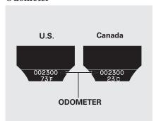
The odometer shows the total distance your vehicle has been driven. It measures miles in U.S. models and kilometers in Canadian models. It is illegal under U.S. federal law and Canadian provincial and territorial regulations to disconnect, reset, or alter the odometer with the intent to change the number of miles or kilometers indicated.
