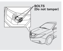
Always keep the radar sensor cover clean. If it gets dirty, clean it with water or a mild detergent. Never use chemical solvents or polishing powder.
