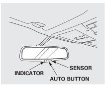
The inside mirror can automatically darken to reduce glare. To turn on this feature, press the button on the bottom of the mirror. The AUTO indicator comes on as a reminder. When it is on, the mirror darkens when it senses the headlights of a vehicle behind you, then returns to normal visibility when the lights are gone. Press the button again to turn off this feature.
