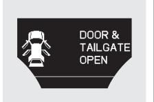
When the tailgate or one or more doors are open, the corresponding indicator for each condition will come on.
