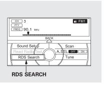
On the FM band selected, you can select the program type provided by the RDS. Press the AUDIO button to display the radio information on the screen. Push down the interface selector, then turn the interface dial to select RDS Search. Press ENTER to set your selection. The principal RDS categories are shown as follows:
