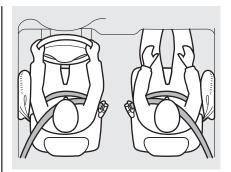
Your vehicle also has side airbags to help protect the upper torso of the driver or a front seat passenger during a moderate to severe side impact (see page 32 for more information on how your side airbags work).
