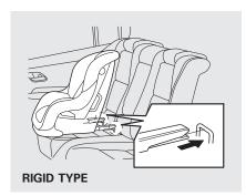
4. Place the child seat on the vehicle seat, then attach the seat to the lower anchors according to the child seat maker's instructions.
