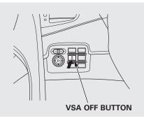
This button is under the driver's side vent. To turn the VSA system on and off, press and hold it until you hear a beep.
