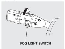
Turn the fog lights on and off by turning the switch next to the headlight switch.
