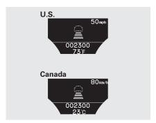
When that vehicle changes lanes or goes out of ACC range, a beeper sounds once. If there is no vehicle ahead of you within ACC range, a dotted-line vehicle icon will be on the multi-information display.
