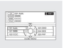
To listen to XM radio, set the power mode to ACCESSORY or ON. Push the ">M > button to select the XM radio. The last channel you listened to will show in the audio screen (if selected) and the center display. Adjust the volume by turning the VOL/ © knob.
