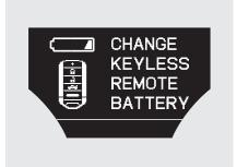
The battery in the remote normally lasts about 2 years. To ensure maximum battery life, do not store the remote close to electrical devices such as computers or TVs. When the multi-information display shows "CHANGE KEYLESS REMOTE BATTERY," replace the battery as soon as possible (see page 191).
