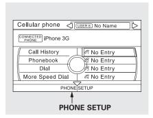
Press the PICK-UP button to go directly to the Cellular Phone screen.
