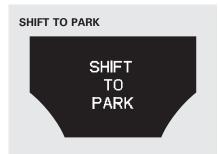
You can only place the vehicle in the VEHICLE OFF (LOCK) mode if the transmission is in Park. You will see the "SHIFT TO PARK" message on the multi-information display if you press the engine start/stop button to turn the vehicle off with the shift lever in any other position except P (Park).
