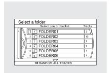
Push the selector up to display the folder list screen, then turn the interface dial to select a folder. Press ENTER to set your selection.
