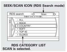
To activate RDS category scan with the interface dial, push the AUDIO button to display the FM radio information on the screen. Push the interface selector down, and turn the interface dial to select RDS search on the audio menu. Press ENTER on the interface selector. The screen shows you the RDS category list.
