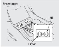
Push the right side of the switch, HI, to rapidly heat up the seat. After the seat reaches a comfortable temperature, select LO by pushing the left side of the switch. This will keep the seat warm.
