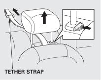
6. Lift the head restraint (see page 162), then route the tether strap through the legs of the head restraint and over the seat-back, making sure the strap is not twisted.
