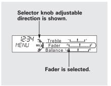
Press the SETUP button to display the sound settings. Turn the selector knob to select an appropriate setting: Bass, Treble, Fader, Balance, Center, Subwoofer, and SVC (speed-sensitive volume compensation). Press the selector (ENTER) knob to enter the setting, then turn the selector knob to adjust the setting.
