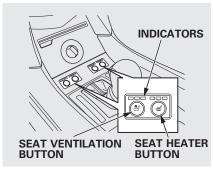
You must select the ON mode by operating the engine start/stop button (see page 194) to use the heaters and the air ventilation system.
