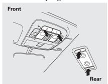
Turn on the front individual map lights by pushing each map light button (\*\*). Push the button again to turn it off. When the door activated position is selected with the light control button, the rear map lights can be turned on by pushing each map light button (\*\*). Push the button again to turn it off.
