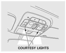
The courtesy lights come on when you turn the parking lights on. To adjust its brightness, press either of the instrument panel brightness control buttons (+ or -) with the ignition switch in the ON (II) position.
