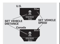
When the speed is set, it is shown along with a vehicle icon and distance bars on the multiinformation display.
