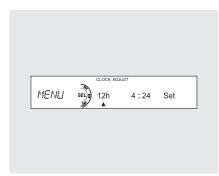
4. Turn the selector knob to select the item which you want to adjust. Turning the selector knob will change the selected item between the clock display setting, hours, minutes, and Set. The selected item is indicated with ▲ in the display.
