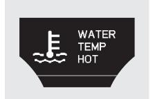
If the pointer of the temperature gauge reaches to or above the red mark, you will also see the "WATER TEMP HOT" message on the multi-information display. This will alert you that the engine should be cooled down.
