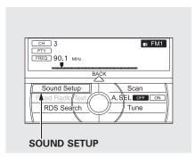
To adjust the sound, press the AUDIO button, push the interface selector down, and turn the interface dial to Sound Setup. Then press ENTER on the interface selector.
