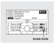
The scan function samples all tracks on the disc in the order they are recorded on the disc.
