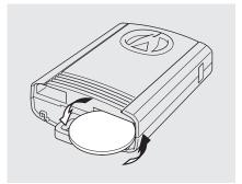
Replace the battery if necessary. Battery type: CR2032
