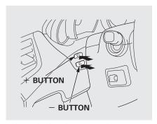
Adjust the brightness of the instrument panel by pressing the + or - button. Press the + button to increase the brightness and the - button to decrease it. The brightness can be set differently for when the headlights are on, and when they are off.
