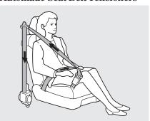
For added protection, the front seat belts are equipped with automatic seat belt tensioners. When activated, the tensioners immediately tighten the belts to help hold the driver and a front passenger in position. The tensioners can be activated during a collision in which the front airbags *do not deploy*. In this case, the airbags would not be needed, but the extra tension in the seat belt could be helpful.
