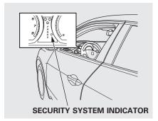
Once the security system is set, opening any door, the tailgate, or the hood without using the key or the remote transmitter/keyless access remote, will cause it to alarm. It also alarms if the audio unit is removed from the dashboard or the wiring is cut.
