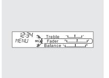
Press the SETUP button to display the audio settings. Turn the selector to select a desired sound mode, then press ENTER to set your selection. Turn the selector to your liking (see page 236 for more sound setting information).
