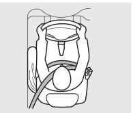
If you ever have a moderate to severe side impact, sensors will detect rapid acceleration and signal the control unit to instantly inflate either the driver's or the passenger's side airbag.
