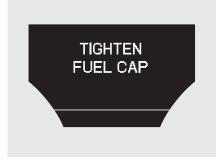
Your vehicle's on board diagnostic system will detect a loose or missing fuel fill cap as an evaporative system leak. The first time a leak is detected a "TIGHTEN FUEL CAP" message appears on the multi-information display. Turn the engine off, and confirm the fuel fill cap is installed. If it is, loosen it, then retighten it until it clicks at least once.
