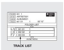
Select a desired folder by turning the interface dial, then press ENTER. The display returns to normal play, and the first track in the selected folder begins to play.
