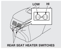
The rear seat heater switches are located under the rear vents. The left (right) switch controls the seat heaters on left (right) outer seating position.
