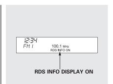
To switch the function between on and off, press and release the TITLE button. With the system on, you will see the "RDS INFO ON" message on the display. If the station you are listening to is an RDS station, the displayed frequency switches to the station name.
