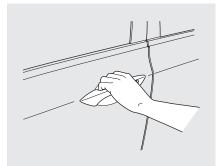
The handle of each front door has a sensor. That sensor works with the remote so you can automatically unlock the door(s).
