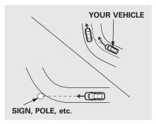
Because of the road condition (curved, winding, etc.) or the state of your vehicle (turning angle, lane position, etc.), CMBS can sometimes mistake a stationary object (light pole, traffic sign, etc.) as a vehicle ahead of you and temporarily operate. This is normal.
