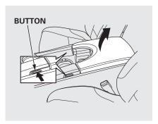
To open the console compartment, push the button on either side of the compartment.
