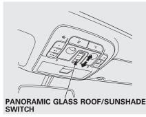
You must turn the ignition switch to the ON (II) position to operate the panoramic glass roof and the sunshades.
