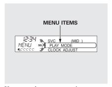
You can select any type of repeat, random and scan modes by using the SETUP button and the selector knob. Push the SETUP button to display the menu items, then turn the selector knob to select "PLAY MODE." Press the selector knob (ENTER) to set the selection.
