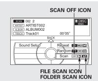
This feature samples all files in the selected folder in the order they are stored. To activate this feature, press the SCAN side of the SCAN/TITLE bar. You can also select the SCAN icon with the interface dial. Push the selector down, turn the dial to select Scan on the AUDIO MENU, then press ENTER. Turn the dial to select the scan icon, then press ENTER. The system begins to play a file for about 10 seconds, and continues to sample the remaining files.
