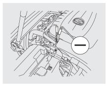
4. Connect the second jumper cable to the negative (-) terminal on the booster battery. Connect the other end to the engine hanger as shown. Do not connect this jumper cable to any other part of the engine.
