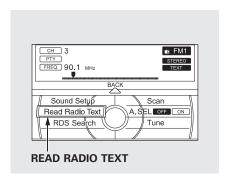
To activate radio text display, use the interface dial. Push the interface selector down, and turn the interface dial to select Read Radio Text. Press ENTER on the interface selector to enter the setting.
