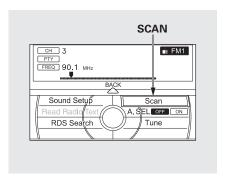
SCAN – The SCAN function samples all stations with strong signals on the selected band. To activate it, press the SCAN side of the SCAN/TITLE bar, then release it.
