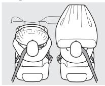
Your vehicle has a supplemental restraint system (SRS) with front airbags to help protect the heads and chests of the driver and a front seat passenger during a moderate to severe frontal collision (see page 28 for more information on how your front airbags work).
