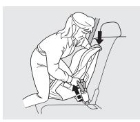
4. After confirming that the belt is locked, grab the shoulder part of the belt near the buckle, and pull up to remove any slack from the lap part of the belt. Remember, if the lap part of the belt is not tight, the child seat will not be secure.
