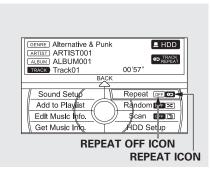
To replay the current track continuously, push the interface selector down during track playback.
