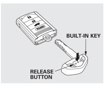
To remove the built-in key, pull it out while pressing the release button. To reinstall the built-in key, push the key into the remote until it clicks.
