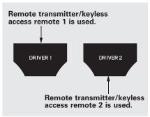
When you turn the ignition switch to the ON (II) position, the display shows "DRIVER 1" or "DRIVER 2" depending on which remote transmitter/keyless access remote you use.
