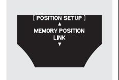
If "MEMORY POSITION LINK" is set to "ON," the driver's seat, the steering wheel, and outside mirror positions move to the position stored in the memory when you open the driver's door, using the remote transmitter.
