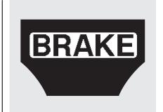
The visual alert is an amber colored BRAKE message that flashes on the multi-information display, the audible alert is a constant beeping sound. If one or more of the alerts come on, take the appropriate means to prevent a collision (apply the brakes, change lanes, etc.).
