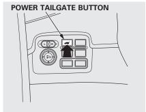
The tailgate can be opened and closed with the remote transmitter/keyless access remote (see page 157 or 189) or the button in the instrument panel when all doors and the tailgate are unlocked.
