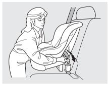
1. With the child seat in the desired seating position, route the belt through the child seat according to the seat maker's instructions, then insert the latch plate into the buckle and remove any slack from the lap portion of the belt.
