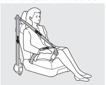
For added protection, the front seat belts are equipped with automatic seat belt tensioners. When activated, the tensioners immediately tighten the belts to help hold the driver and a front passenger in position. The tensioners can be activated during a collision in which the front airbags *do not deploy*. In this case, the airbags would not be needed, but the extra tension in the seat belt could be helpful.
