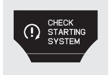
If there is a problem with the starting system, you will see a "CHECK STARTING SYSTEM" message on the multi-information display when the ignition switch is turned to the ON (II) position. You will also see this message when the auto control mode of the starting system has a problem.
