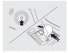
To turn the vehicle off, make sure the vehicle is completely stopped, shift to Park (P), then press the engine start/stop button. The engine stops and the power mode switches from ON to VEHICLE OFF (LOCK).
