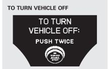
You will also see the "TO TURN VEHICLE OFF:" message on the multi-information display. Press the engine start/stop button twice to change the power mode from ACCESSORY to VEHICLE OFF (LOCK).
