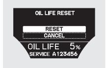
4. Select "RESET" by pressing the INFO (▲/▼) button, then press the SEL/ RESET button to reset the engine oil life display. The maintenance item code(s) will disappear, and the engine oil life will reset to "100." If you want to cancel the oil life reset mode, select "CANCEL."
