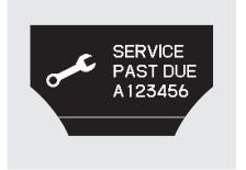
If the indicated maintenance service is not done and the remaining engine oil life reaches 0%, the multi-information display will show the message "SERVICE PAST DUE" and the maintenance item code(s). This message is displayed when the total distance traveled is less than 10 miles (for U.S. models) or 10 km (for Canadian models) after the engine oil life became 0%.
