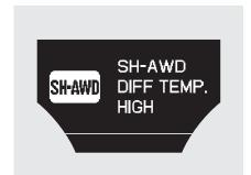
If the SH-AWD indicator blinks while driving, it indicates the differential temperature is too high. You will also see an "SH-AWD DIFF TEMP. HIGH" message on the multi-information display. If this happens, pull to the side of the road when it is safe, shift to Park, and let the engine idle until the indicator goes out. If the indicator does not go out, take your vehicle to a dealer to have it checked.
