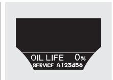
Press the SEL/RESET button on the steering wheel repeatedly to select the engine oil life. The message "SERVICE," along with "0%," and the maintenance item code are displayed on the multi-information display when the calculated engine oil life is 0 to 1 percent.
