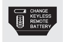
The battery in the remote normally lasts about 2 years. To ensure maximum battery life, do not store the remote close to electrical devices such as computers or TVs. When the multi-information display shows "CHANGE KEYLESS REMOTE BATTERY," replace the battery as soon as possible (see page 191).
