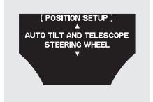
When "AUTO TILT AND TELESCOPE STEERING WHEEL" is set to "ON," the steering wheel automatically moves fully up when you turn the ignition switch to the LOCK (0) position and remove the key (or the vehicle is in VEHICLE OFF mode on models with keyless access system).
