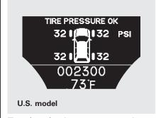
To select the tire pressure monitor, press the INFO button several times with the ignition switch in the ON (II) position.
