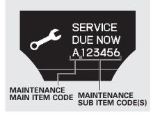
When the remaining oil life is 5 to 1 percent, the multi-information display shows a "SERVICE DUE NOW" message with the same maintenance items "SERVICE DUE SOON" was displayed with. When you see this message, have the indicated maintenance performed as soon as possible.
