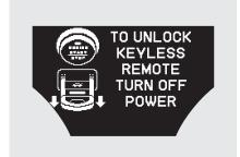
When the keyless access system main switch in the glove box is off, the "TO UNLOCK KEYLESS REMOTE TURN OFF POWER" message will be shown after shifting into Park.
