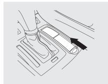
Your vehicle has two accessory power sockets. One is next to the shift lever. The other is in the console compartment.
