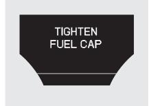
Your vehicle's on board diagnostic system will detect a loose or missing fuel fill cap as an evaporative system leak. The first time a leak is detected a "TIGHTEN FUEL CAP" message appears on the multi-information display. Turn the engine off, and confirm the fuel fill cap is installed. If it is, loosen it, then retighten it until it clicks at least once.
