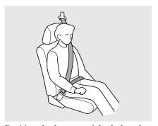
Position the lap part of the belt as low as possible across your hips, then pull up on the shoulder part of the belt so the lap part fits snugly. This lets your strong pelvic bones take the force of a crash and reduces the chance of internal injuries. If necessary, pull up on the belt again to remove any slack, then check that the belt rests across the center of your chest and over your shoulder.
