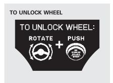
If the steering wheel is locked, the engine cannot start. The multi-information display shows you the above message and the indicator in the engine start/stop button blinks. To unlock the steering wheel, apply force by turning it left and right while pressing the engine start/stop button at the same time.
