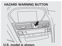
Push the button between the center vents to turn on the hazard warning lights (four-way flashers). This causes all four outside turn signals and both indicators in the instrument panel to flash. Use the hazard warning lights if you need to park in a dangerous area near heavy traffic, or if your vehicle is disabled.
