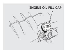
Unscrew and remove the engine oil fill cap on top of the valve cover. Pour in the oil slowly and carefully so you do not spill. Clean up any spills immediately. Spilled oil could damage components in the engine compartment.
