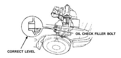
5-SPEED TRANSMISSION OIL CHANGE CAPACITY: 1.9  $\ell$  (1.7 Imp qt, 2.0 US qt).
