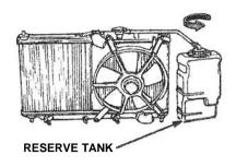
CAUTION: Radiator coolant will damage paint. Quickly rinse any spilled coolant from painted surfaces.
