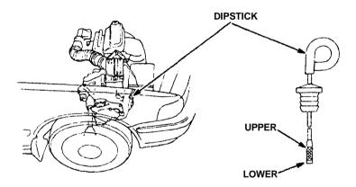
Insert the dipstick, remove it again, and read the fluid level. The fluid level should be between the upper and lower marks.
