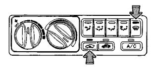
For extra door window defrosting or defogging, select either the , or function, switch to the setting, and turn the fan on.
