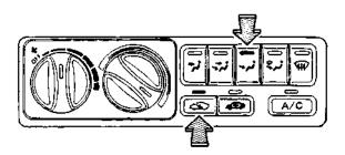
To warm up the interior quickly, push in the button so the inside air will be recirculated to the heater.
