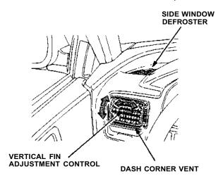
After the windows are defrosted, you may wish to retain the mode for more comfort. Turning the temperature control dial counterclockwise will reduce the temperature of the air exiting the dash corner vents without appreciably affecting the heat to your leg and foot area. Continue to adjust the temperature and fan speed to find the most comfortable setting.
