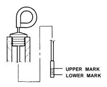
5. If the level is below the lower mark, add fluid to bring it to the upper mark. Always use Honda Premium Formula Automatic Transmission Fluid (ATF). If it is not available, you may use a Dexron III automatic transmission fluid as a temporary replacement. However, continued use can affect shift quality. Have the transmission drained and refilled with Honda ATF as soon as it is convenient. 2.3CL — Add fluid in the dipstick tube. 3.0 CL — Remove the fill plug to add fluid.
