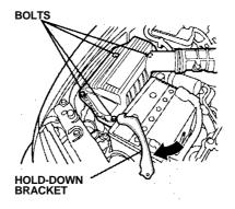
Loosen the four bolts, then remove the air cleaner housing cover.  Remove the old air cleaner element. Clean the inside of the housing with a damp rag.
