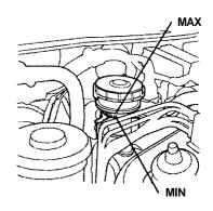
Low fluid level can indicate a leak in the clutch system. Have this system inspected as soon as possible.
