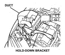
Loosen the nuts on the battery hold-down bracket. Remove the bracket.
