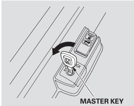
To protect items in the trunk when you need to give the key to someone else, lock the trunk release handle with the master key and give the other person the valet key.
