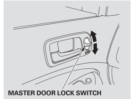
The master door lock switch allows control of all door locks from the driver's door. Push the switch down to lock all doors, and up to unlock them.
