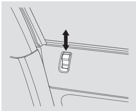
Each door has a lock tab at the top of the door. When you push down the lock tab on the driver's door, all doors lock. Pulling up the lock tab on the driver's door only unlocks that door. The lock tab on each passenger's door only locks and unlocks that door.
