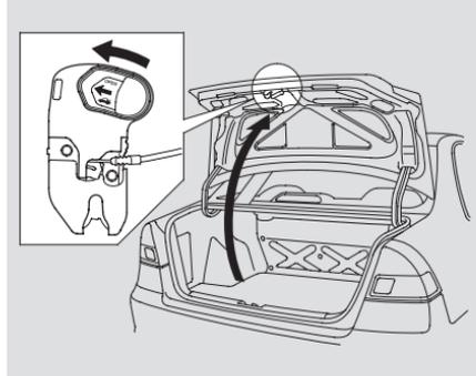
As a safety feature, your car has a release lever on the trunk latch so the trunk can be opened from the inside.
