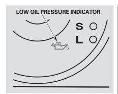
This indicator should light when the ignition switch is ON (II), and go out after the engine starts. It should never come on when the engine is running. If it starts flashing, it indicates that the oil pressure dropped very low for a moment, then recovered. If the indicator stays on with the engine running, it shows that the engine has lost oil pressure and serious engine damage is possible. In either case, you should take immediate action
