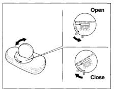
When the remote transmitter's battery begins to get weak, it may take several pushes on the buttons to lock or unlock the doors, and the LED will get dim. Replace the battery as soon as possible.
