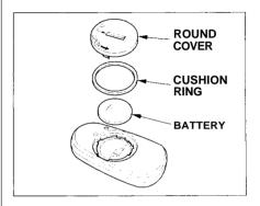
To replace the battery, remove the round cover on the back of the transmitter by turning it counter-clockwise with a quarter coin.
