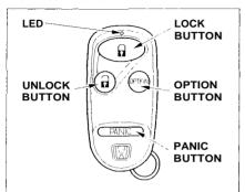
On EX model in the U.S. You can lock and unlock your car with the remote transmitter. When you push the Lock button, both doors will lock.
