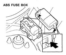
Vehicles equipped with ABS have a third fuse box for the ABS. It is in the engine compartment on the passenger's side.
