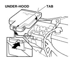
All the electrical circuits in your vehicle have fuses to protect them from a short circuit or overload These fuses are located in two or three fuse boxes.
