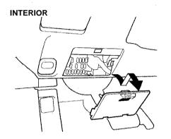
The interior fuse box is underneath the dashboard on the driver's side. Remove the fuse box lid by swinging the lid down and pulling it straight out of its hinges.
