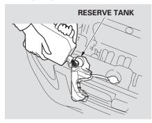
If the coolant level in the reserve tank is at or below the MIN line, add coolant to bring it up to the MAX line. Inspect the cooling system for leaks. The coolant you add should always be a mixture of 50 percent antifreeze and 50 percent water. Never add straight antifreeze or plain water.
