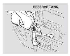
The coolant level should be up to the base of the filler neck. Add coolant if it is low.
