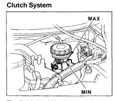
The fluid should be between the MIN and MAX marks on the side of the reservoir. If it is not, add brake fluid to bring it up to that level. Use the same DOT3 or DOT4 brake fluid from a sealed container specified for the brake system.
