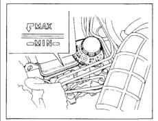
The fluid should be between the MIN and MAX marks on the side of the reservoir. If it is at or below the MIN mark, it may indicate a problem in the braking system. Have the dealer inspect your car. If the fluid level is half an inch or more above the MAX mark, it may indicate a problem in the ABS. Have your dealer inspect the system as soon as possible.
