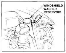
Check the level in the windshield washer reservoir at least monthly during normal usage. In bad weather, when you use the washers often, check the level every time you stop for fuel.
