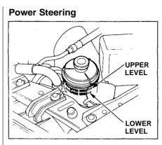
You should check the fluid level in the power steering reservoir monthly. Check the level when the engine is cold. Look at the side of the reservoir. The fluid should be between the UPPER LEVEL and LOWER LEVEL. If it is below the LOWER LEVEL, add power steering fluid to the UPPER LEVEL.
