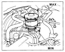
The fluid should be between the MIN and MAX marks on the side of the reservoir. If the level is at or below the MIN mark, it is an indication that your brake system needs attention. Have the brake system inspected for leaks or worn brake pads. If you add brake fluid to bring it up to the MAX mark, use Genuine Honda Brake Fluid or an equivalent from a sealed container that is marked DOT3 or DOT4 only. Brake fluid marked DOT5 is not compatible with your car's braking system.
