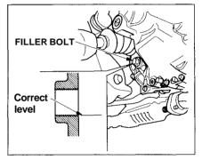
Check the oil level a couple of minutes after shutting off the engine. Make sure the car is on level ground. Remove the transmission filler bolt. The oil level should be up to the edge of the bolt hole. Feel inside the bolt hole with your finger. If you do not feel any oil, slowly add oil until it starts to run out of the hole. Reinstall the filler bolt and tighten it securely. Only use an API Service SF or SG grade motor oil with a viscosity of SAE 10W-30 or 10W-40.
