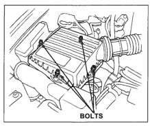
The air cleaner element is inside the box on the passenger's side of the engine compartment. To replace it:
