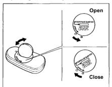
When the remote transmitter's battery begins to get weak, it may take several pushes on the button to lock or unlock the doors, and the LED will get dim. Replace the battery as soon as possible.
