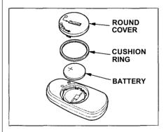
To replace the battery, remove the round cover on the back of the transmitter by turning it counterclockwise with a coin.
