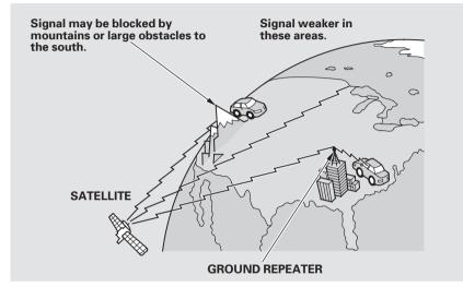
The XM satellites are in orbit over the equator; therefore, objects south of the vehicle may cause satellite reception interruptions. To help compensate for this, ground-based repeaters are placed in major metropolitan areas. Satellite signals are more likely to be blocked by tall buildings and mountains the farther north you travel from the equator.
