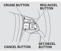
1. Push the CRUISE button on the steering wheel. The CRUISE MAIN indicator on the instrument panel comes on.
