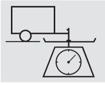
• Tongue Load: The weight that the tongue of a fully-loaded trailer puts on the hitch should be approximately 10% of the total trailer weight. Too much tongue load reduces front-tire traction and steering control. Too little tongue load can make the trailer unstable and cause it to sway.
