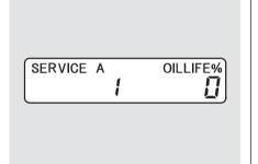
When the remaining engine oil life is 0 percent, the engine oil life indicator will blink. The display comes on every time you turn the ignition switch to the ON (II) position. The Maintenance Minder indicator ( ) also comes on and remains on in the instrument panel. When you see this message, immediately have the indicated maintenance done by your dealer.
