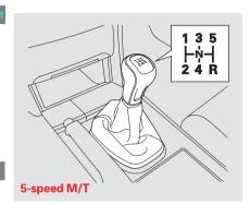
On models with 5-speed manual transmission. or models with 6-speed manual transmission The manual transmission is synchronized in all forward gears for smooth operation. It has a lockout so vou cannot shift directly from fifth to reverse.
