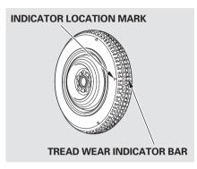
Replace the tire when you can see the tread wear indicator bars. The replacement tire should be the same size and design, mounted on the same wheel. The spare tire is not designed to be mounted on a regular wheel, and the spare wheel is not designed for mounting a regular tire.
