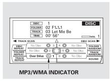
Using the interface selector, you can see the list of all the files and folders within a disc. While playing a MP3/ WMA disc, press the AUDIO button. The currently playing folder and file information comes on the screen.
