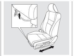
To adjust the seat forward or backward, pull up on the bar under the seat cushion's front edge. Move the seat to the desired position, and release the bar. Try to move the seat to make sure it is locked in position.
