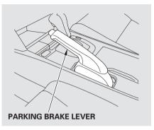
To apply the parking brake, pull the lever up fully. To release it, pull up slightly, push the button, and lower the lever. The parking brake indicator on the instrument panel should go out when the parking brake is fully released (see page 57).
