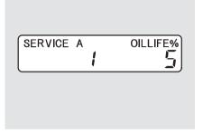
When the remaining engine oil life is 5 to 1 percent, you will see a "SERVICE" message along with the same maintenance item code(s), every time you turn the ignition switch to the ON (II) position.
