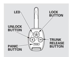
LOCK — Press this button once to lock both doors. Some exterior lights will flash once. When you push LOCK twice within 5 seconds, you will hear a beep to verify that the doors are locked and that the security system has set. You cannot lock the doors if either door is not fully closed or the key is in the ignition switch.
