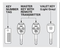
The master key fits all the locks on your vehicle. The valet key works only in the ignition and the driver's door lock. You can keep the trunk release handle, and glove box locked when you leave your vehicle and the valet key at a parking facility.
