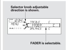
Press the MENU button to display the sound settings. Turn the selector knob to select an appropriate setting: bass, treble, fader, balance, SUBW\* (subwoofer) and SVC (speedsensitive volume compensation). Press the selector knob (ENTER) to enter the setting, then turn the selector knob to adjust the setting.
