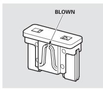
5. Look for a blown wire inside the fuse. If it is blown, replace it with one of the spare fuses of the same rating or lower.
