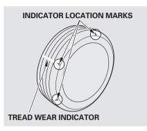
Your tires have wear indicators molded into the tread. When the tread wears down, you will see a 1/2 inch (12.7 mm) wide band across the tread. This shows there is less than 1/16 inch (1.6 mm) of tread left on the tire.
