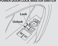
To lock both doors, push the front of the master door lock switch on either door, pull the lock tab rearward on the driver's door, or use the key on the outside lock on the driver's door
