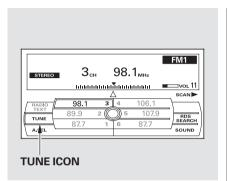
TUNE — Use the TUNE bar to tune the radio to a desired frequency. Press the right side of the bar to tune to a higher frequency, or the left side to tune to a lower frequency. To tune with the interface dial, push the selector down, and turn the knob to the TUNE icon. Then press ENTER on the selector, and turn the knob to the desired frequency. To exit the TUNE mode, press ENTER on the selector, then push the selector up.
