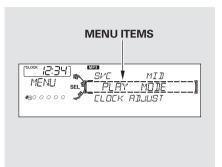
You can select any type of repeat, random and scan modes by using the MENU button and the selector knob. Push the MENU button to display the menu items, then turn the selector knob to select "PLAY MODE." Press the selector knob (ENTER) to set the selection.
