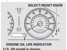
To see the current engine oil life, turn the ignition switch to the ON (II) position, then press and release the select/reset knob repeatedly until the engine oil life indicator appears (see page 64).
