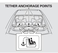
A child seat with a tether can be installed in any seating position in the back seat, using one of the anchorage points shown above.
