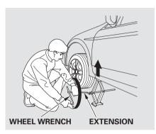
9. Use the extension and the wheel nut wrench as shown to raise the vehicle until the flat tire is off the ground.
