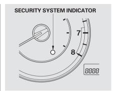
Once the security system sets, opening either door, the trunk, or hood without using the key or the remote transmitter, will cause the alarm to activate. It also activates if the ignition switch is turned to the ON (II) position, the audio unit is removed from the dashboard, or the wiring is cut.
