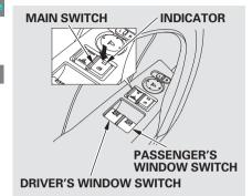
Turn the ignition switch to the ON (II) position to raise or lower either window. To open a window, push the switch down and hold it. Release the switch when you want the window to stop. Pull back on the switch and hold it to close the window.
