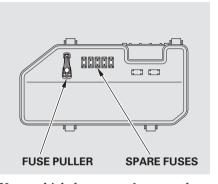
Your vehicle has spare fuses on the back of the under-hood fuse box cover.
