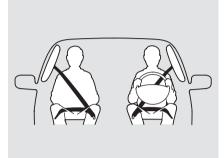
In addition, your vehicle has side curtain airbags to help protect the heads of the driver, front passenger, and passengers in the outer rear seating positions during a moderate to severe side impact (see page 29 for more information on how your side curtain airbags work).
