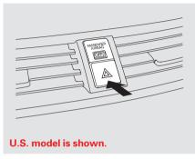
Push the button between the center vents to turn on the hazard warning lights (four-way flashers). This causes all four outside turn signals and both turn indicators in the instrument panel to flash. Use the hazard warning lights if you need to park in a dangerous area near heavy traffic, or if your vehicle is disabled.
