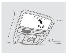
To open the sunglasses holder, push then release the indent. It will unlatch and swing down. To close it, push it until it latches. Make sure the holder is closed while you are driving.
