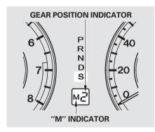
When you move the shift lever from "D" to "S" and pull either paddle shifter, the gear position indicator displays "M" along with the selected gear number.
