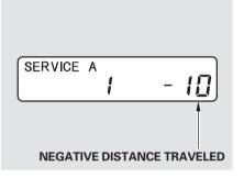
If you do not perform the indicated maintenance, negative distance traveled is displayed and begins to blink after the vehicle has been driven 10 miles (10 km) or more.
