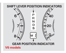
Using a paddle shift mode, the gear position indicator shows you the selected gear number (see page 315).
