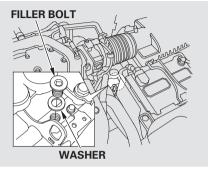
If no fluid comes out, remove the filler bolt and washer. Slowly add Honda Manual Transmission Fluid (MTF) until it starts to run out of the check bolt hole.
