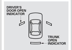
The appropriate indicator comes on if the trunk or either door is not closed tightly.
