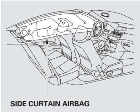
In a moderate to severe side impact, sensors will detect rapid acceleration and signal the control unit to instantly inflate the side curtain airbag.
