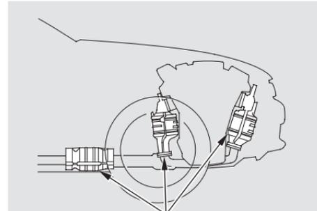
**THREE WAY CATALYTIC CONVERTERS**
