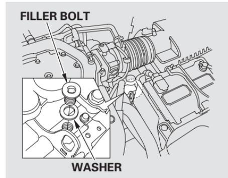
If no fluid comes out, remove the filler bolt and washer. Slowly add Honda Manual Transmission Fluid (MTF) until it starts to run out of the check bolt hole.
