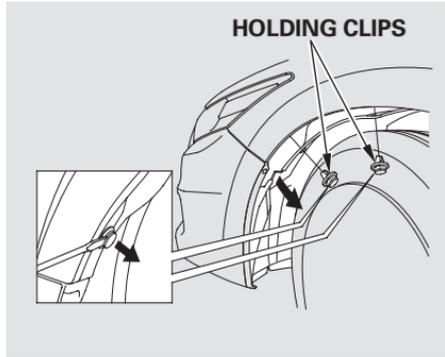
1. To change the bulb on the driver's side, start the engine, turn the steering wheel all the way to the right, then turn off the engine. To change the bulb on the passenger's side, turn the steering wheel to the left.
