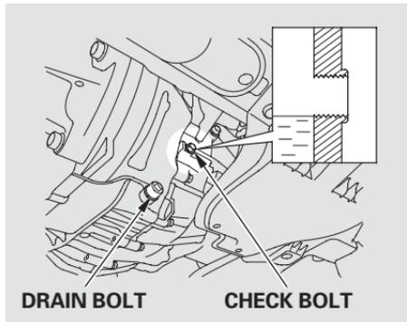
Remove the check bolt and look for transmission fluid coming out of the bolt hole. If a small amount of fluid drips out of the bolt hole, reinstall the check bolt.
