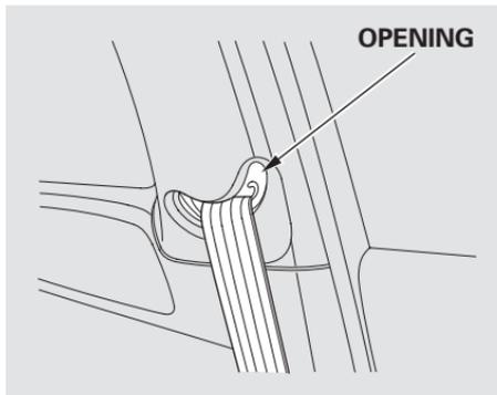
Dirt build-up around the openings of the seat belt anchors can cause the belts to retract slowly. Wipe the openings with a clean cloth dampened in mild soap and warm water or isopropyl alcohol.
