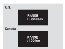
When you press the INFO ( $\checkmark$ ) button, the display changes as shown above. This is the estimated distance you can travel on the fuel remaining in the tank. This distance is estimated from the fuel economy you received over the last several miles (kilometers), so it will vary with changes in speed, traffic, etc. It measures miles in U.S. models and kilometers in Canadian models.
