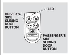
To open and close a power sliding door, press and hold the appropriate button for at least 1 second. If you forget to unlock the door, you will hear three beeps. Unlock the door, and try again.
