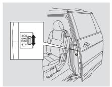
The childproof door locks are designed to prevent children seated in the rear from accidentally opening the rear sliding doors. Each door has a lock lever near the edge. With the lever in the LOCK position, the door cannot be opened from the inside regardless of the position of the lock tab. To open the door, pull the lock tab up and use the outside door handle.
