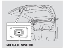
The tailgate can also be closed by pressing the button on the tailgate. If you press the button again while the tailgate is closing, you will hear three beeps, and the tailgate will stop moving, reverse direction, and stop at the fully opened position.
