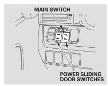
The dashboard switches to the left of the steering column allow you to open or close the power sliding doors.
