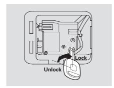
On LX, EX and EX-L models Use the key to unlock the tailgate as shown, then pull the outer handle to open the tailgate.
