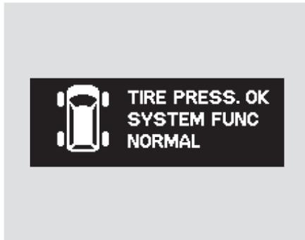
To display the tire pressure monitor, press the INFO button until it appears on the multi-information display.
