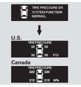
When the tire pressure monitor is shown on the multi-information display, press the SEL/RESET button. The display changes as shown.
