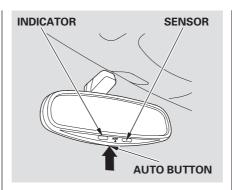
The inside mirror can automatically darken to reduce glare. To turn on this feature, press the button on the bottom of the mirror. The AUTO indicator comes on as a reminder. When it is on, the mirror darkens when it senses the headlights of a vehicle behind you, then returns to normal visibility when the lights are gone. Press the button again to turn off this sensing.
