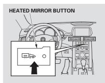
The outside mirrors are heated to remove fog and frost. With the ignition switch in the ON (II) position, turn on the heaters by pressing the button. The indicator in the button comes on as a reminder. Press the button again to turn the heaters off. Pressing this button also turns the rear window defogger on and off
