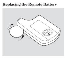
Replace the batteries if necessary. Battery type: CR2025
