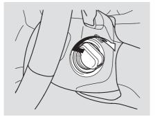
When you push the ignition switch, the remote and the vehicle recognize each other. After the recognition, the remote indicator flashes, and a beeper sounds once. After the beep, turn the ignition switch. When the remote is out of the
