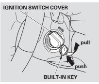
To remove the ignition switch cover, insert the built-in key (see page 173), then pull the cover out by pulling the built-in key while pushing it.
