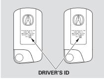
When you unlock the door with your remote, each remote activates the keyless memory settings related to that remote. The driver's ID (Driver 1 or Driver 2) is shown on the back of each remote. Here are the settings activated with the remote;
