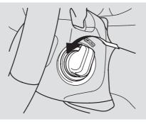
To turn the ignition switch to the LOCK (0) position, put the transmission in Park, press the switch in, and turn it to the LOCK (0) position. When the transmission is not in Park, you cannot turn the ignition switch to the LOCK (0) position.
