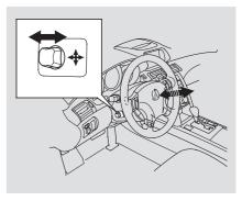
Release the switch when the steering wheel reaches the desired position. Make sure the steering wheel points towards your chest, not toward your face, and that you can see the instrument panel gauges and indicators.
