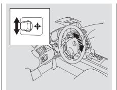
Move the steering wheel in, out, up, or down by pushing and holding the adjustment switch in that direction.
