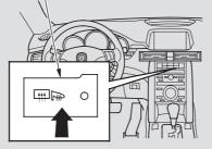
The rear window defogger clears fog, frost, and thin ice from the window. Push the defogger button to turn it on and off. Pushing this button also turns the mirror heaters on and off. The indicator in the button comes on to show the defogger is on. If you do not turn it off, the defogger will shut itself off after 5 to 40 minutes (depending on the ambient temperature). It also shuts off when you turn off the ignition switch. You have to turn it on again when you restart the vehicle.
