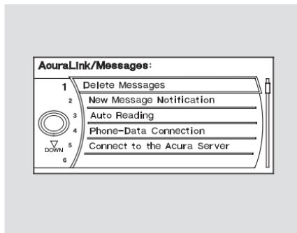
To access the following functions, press the SETUP button, push the interface selector to the right to select MORE, then rotate the interface knob to select AcuraLink/ Messages.
