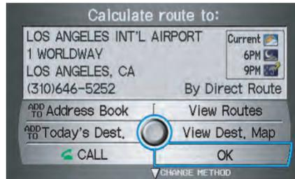
Say or select **OK**. The system calculates the route using the method shown on the screen (see *Map Screen* on page 55).
