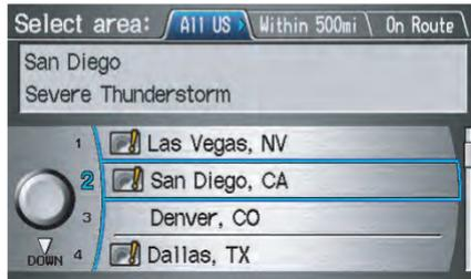
You can view three types of lists by selecting a sorting method from “All US,” “Within 500mi,” or “On Route.” A warning icon in the list indicates that your vehicle is in the warning area, or the calculated route runs through the area. When you select a listed item by pushing in on the **Interface Dial**, the detailed information will be displayed.
