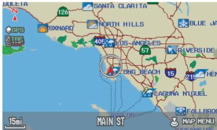
When you scroll through the map using the **Interface Dial**, the weather icon is displayed at the top right of the screen. This shows you the weather at the cursor position.
