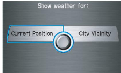
When you select **Current Position**, the Forecast screen will be displayed. When you select **City Vicinity**, the Enter city name screen will be displayed. Enter the name of the city using the **Interface Dial**. If the system does not find an exact match, select **LIST** when you finish entering the name of the city. Select a desired city from the list. The Forecast screen will be displayed.
