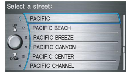
After you have completed the first street name, the display changes to the **Enter intersecting street** screen. Enter the name of the other intersecting street by saying the item number, or selecting the item number using the **Interface Dial**.
