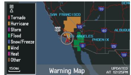
Select the colored area by moving the **Interface Dial** left, right, up, or down. If desired, rotate the **Interface Dial** to change the map scale (15, 50, or 150 miles). When you have the crosshairs in the desired area, push in on the **Interface Dial**. The *Weather Warning* screen will be displayed.
