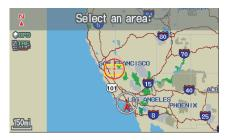
Use the **Interface Dial** to move the crosshairs to the area of the state close to your intended destination. If desired, rotate the **Interface Dial knob** to change the map scale. When you have the crosshairs in the desired area, push in on the **Interface Dial**. The address of the location you have selected will appear at the top of the screen.
