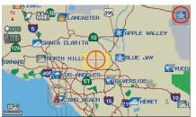
When you select the weather icon next to a city name and push in the **Interface Dial**, the Forecast screen will be displayed. To return to the map screen, press the **CANCEL** button or move the **Interface Dial** to the left.
