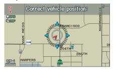
Use the Interface Dial to move the vehicle position arrowhead to the correct location, and push in on the Interface Dial. The display will change to:
