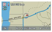
The map screen starts displaying a series of dots (breadcrumbs) to show the path you have taken if **Off-road Tracking** on the SETUP screen (Other) is set to **ON** (see page 112).
