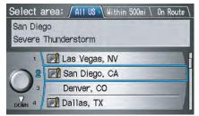
You can view three types of lists by selecting a sorting method from "All US," "Within 500mi," or "On Route." A warning icon in the list indicates that your vehicle is in the warning area, or the calculated route runs through the area. When you select a listed item by pushing in on the **Interface Dial**, the detailed information will be displayed.
