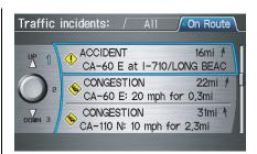
Select an incident from the list, and push in on the **Interface Dial** twice. The system will read the incident information, displaying the confirmation screen:
