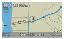
The map screen starts displaying a series of dots (breadcrumbs) to show the path you have taken if **Off-road Tracking** on the SETUP screen (Other) is set to **ON** (see page 112). By following the dots, you can backtrack to the mapped road you originally left.
