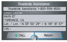
An Acura Roadside Assistance number is provided as a courtesy to Acura clients. If you have a paired Bluetooth phone and it is on, then you can call Acura Roadside Assistance by using your system. Select **CALL** by voice or by using the **Interface Dial**, and then select **Yes** on the confirmation screen.
