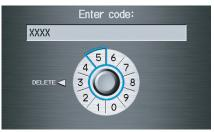
Enter the four-digit security code. If you have entered it correctly, the display changes to the **Disclaimer** screen. If you make a mistake, the system will display "INCORRECT PIN." Re-enter your 4-digit security code. You have 10 chances to enter the correct code. If all 10 are incorrect, turn the ignition to OFF, then back to ON (II) to have 10 more chances to enter the correct code.
