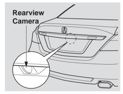
Whenever you shift to R (Reverse) with the ignition switch in the ON (II) position, the rear view is shown on the navigation screen. For the best image, always keep the rearview camera lens clean, and be sure it is not covered.
