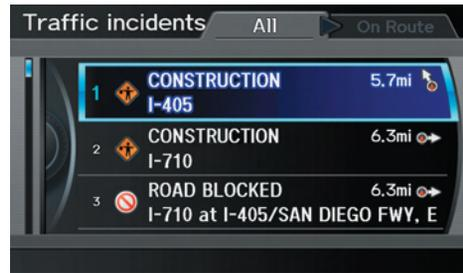
When you select the “All” tab, a list of all incidents within 200 miles from the vehicle’s location will be displayed. When you select the “On Route” tab, a list of all incidents on the current route within 200 miles from the vehicle’s location will be displayed. Incidents are listed by distance from your current position outward in all directions.
