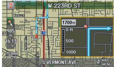
On the map screen, the location of the maneuver is marked with a small yellow square. The guidance window is simply an enlargement of the next maneuver area. After you complete the maneuver, the display returns to a full map screen when single-screen mode is set, or to a map and direction list screen when split-screen mode is set.
