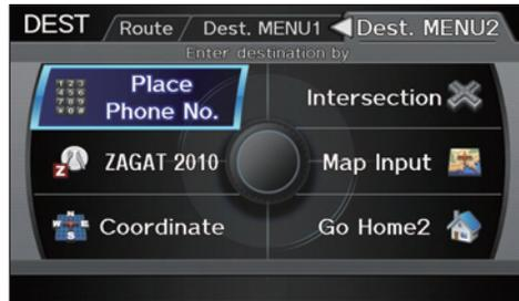
To display the “Dest. MENU 1” tab or the “Dest. MENU 2” tab, move the **Interface Dial** to the left or right.
