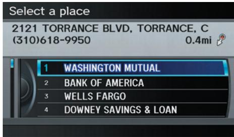
The distance and direction to the destination at the cursor position in the list are shown on the screen. The distance shown is straight line distance (as the crow flies), not driving distance. Say or select the number (1-4) of the desired destination from the list.
