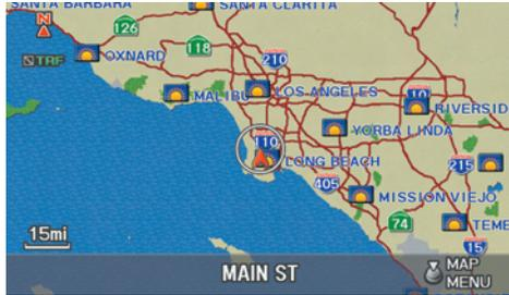
When you scroll through the map using the **Interface Dial**, the weather icon is displayed at the top right of the screen. This shows you the weather at the cursor position.
