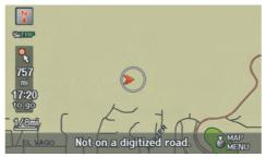
The map screen starts displaying a series of dots (breadcrumbs) to show the path you have taken if **Off-road Tracking** on the SET UP screen (Other) is set to **ON** (see page 117).
