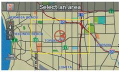
The red arrow indicates your vehicle position. Find your desired destination by moving the **Interface Dial** up and down and to the left and right. The map and crosshairs will move in the same direction.
