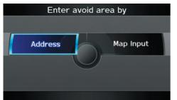
Either select **Address** or **Map Input** on the Enter avoid area by screen. Each choice provides a slightly different way to locate the approximate map display for drawing the area you wish to avoid. After selecting the choice, a map screen will be displayed.
