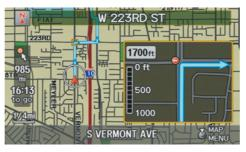
On the map screen, the location of the maneuver is marked with a small yellow square. The guidance window is simply an enlargement of the next maneuver area. After you complete the maneuver, the display returns to a full map screen when single-screen mode is set, or to a map and direction list screen when splitscreen mode is set.
