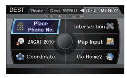
To display the "Dest. MENU 1" tab or the "Dest. MENU 2" tab, move the **Interface Dial** to the left or right.
