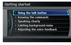
Select the line number of the desired tutorial you want to view, and the tutorial will automatically be read. To stop the reading, push in on the **Interface Dial** and select **STOP**. To resume the reading, push in on the **Interface Dial** again.
