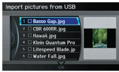
Rotate the **Interface Dial** knob and select the images to be uploaded to the HDD. Move the **Interface Dial** down and select **OK**.
