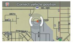
4. Rotate the **Interface Dial knob** so the vehicle position arrowhead is pointing in the correct direction, and push in on the **Interface Dial**. The display will return to the previous screen.
