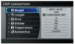
3. Rotate the **Interface Dial knob** to select the type of unit you want to convert (for example, weight) and push in on the **Interface Dial** to select. The screen for that conversion type appears (see illustration in step 4).
