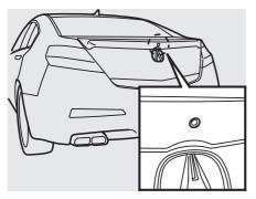
When you shift to R (Reverse) with the power mode in the ON mode, the rear view is shown on the navigation screen. Parking guidelines appear in the rear view. For the best image, always keep the rearview camera lens clean, and be sure it is not covered.
