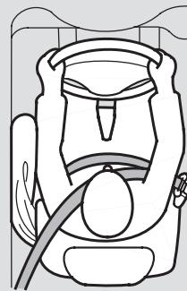
If you ever have a moderate to severe side impact, sensors will detect rapid acceleration and signal the control unit to instantly inflate either the driver's or the passenger's side airbag.
