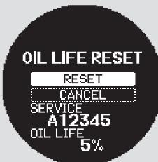
4. Select "RESET" by pressing the INFO ( $\blacktriangle/\blacktriangledown$ ) button, then press the SEL/RESET button to reset the engine oil life display. The maintenance item code(s) will disappear, and the engine oil life will reset to "100." If you want to cancel the oil life reset mode, select "CANCEL."
