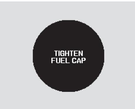
Your vehicle's on board diagnostic system will detect a loose or missing fuel fill cap as an evaporative system leak. The first time a leak is detected a "TIGHTEN FUEL CAP" message appears on the multi-information display.
