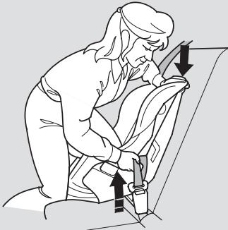
4. After confirming that the belt is locked, grab the shoulder part of the belt near the buckle, and pull up to remove any slack from the lap part of the belt. Remember, if the lap part of the belt is not tight, the child seat will not be secure.
