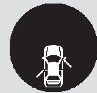
When one or more doors or the trunk lid are not tightly closed, the corresponding indicator for each condition will come on.
