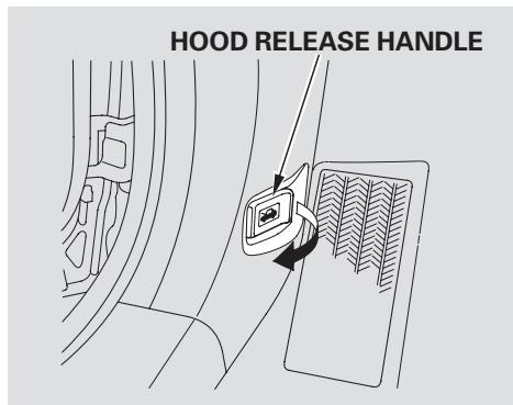
1. Park the vehicle, and set the parking brake. Pull the hood release handle located under the lower left corner of the dashboard. The hood will pop up slightly.
