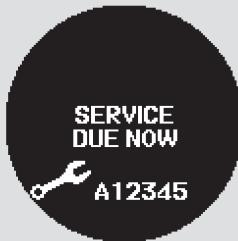
When the remaining oil life is 5 to 1 percent, the multi-information display shows a "SERVICE DUE NOW" message with the same maintenance items "SERVICE DUE SOON" was displayed with. When you see this message, have the indicated maintenance performed as soon as possible.
