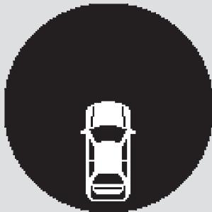
When the trunk is not tightly closed, this indicator will come on.
