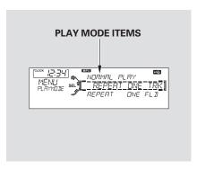
**REPEAT ONE TRK** — This feature continuously plays a file. Select normal play to turn it off. Pressing either side of the SKIP bar also turns off this feature.
