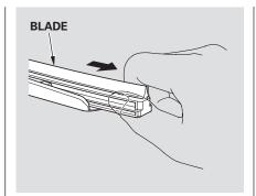
3. Remove the blade from its holder by grabbing the tabbed end of the blade. Pull firmly until the tabs come out of the holder. 4. Examine the new wiper blades. If they have no plastic or metal reinforcement along the back edge, remove the metal reinforcement strips from the old wiper blade, and install them in the slots along the edge of the new blade.
