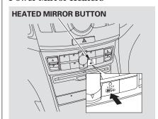
The outside mirrors are heated to remove fog and frost. With the ignition switch in the ON (II) position, turn on the heaters by pressing the rear window defogger button. The indicator in the button comes on as a reminder. Press the button again to turn the heaters and the defogger off.
