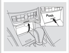
On vehicles without navigation system To open the center pocket, push on the lid. It will unlatch and swing up. To close it, push the lid down until it latches.
