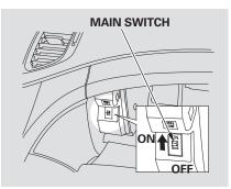
To protect items in the trunk, you can disable the trunk release button on the driver's door and the trunk release switch on the trunk lid by turning off the trunk main switch in the glove box and locking the glove box. Make sure either rear seat is not folded down.
