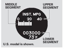
The multi-information display consists of an upper segment, a middle segment and a lower segment. In the normal display mode, the upper and middle segments display trip computer information, such as fuel economy or average speed. The lower segment displays the odometer/trip meter (A/B), outside temperature, and engine oil life and maintenance item code(s).
