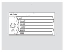
Push ENTER on the selector to display the items on that list, then turn the knob on the interface dial to select a desired list. Pushing the selector up or down moves a selection to the top or bottom of the screen items. Press ENTER to set your selection.
