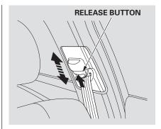
The front seats have adjustable seat belt anchors. To adjust the height of an anchor, press and hold the release button and slide the anchor up or down as needed (it has four positions). Never place the shoulder portion of a lap/shoulder belt under your arm or behind your back. This could cause very serious injuries in a crash.
