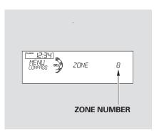
5. Once the correct zone is displayed, press the selector knob. The display then returns to normal.
