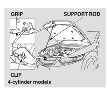
3. *4-cylinder models*Holding the grip, pull the support rod out of its clip. Insert the end into the designated hole in the hood marked by an arrow.
