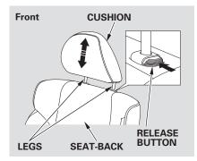
Adjusting the Head Restraint
