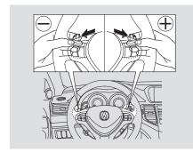
To shift up or down, use the + (right) or — (left) paddle shifter on either side of the steering wheel.
