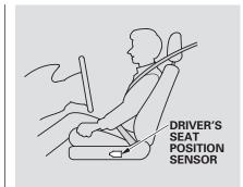
The driver's advanced front airbag system includes a seat position sensor under the seat. If the seat is too far forward, the airbag will inflate with less force, regardless of the severity of the impact.
