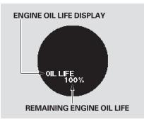
To see the current engine oil life displayed on the multi-information display, turn the ignition switch to the ON (II) position, and press the SEL/RESET button on the steering wheel repeatedly until the engine oil life is displayed.
