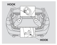
Cargo hook buttons in the trunk can be used to install a net for securing items.
