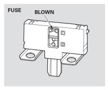
3. Check each of the large fuses in the under-hood fuse box by looking at the wire inside. Removing these fuses requires a Phillips-head screwdriver.
