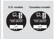
Adjust the outside temperature value by pressing the INFO (▲/▼) button repeatedly. Press the SEL/RESET button to set the desired value.
