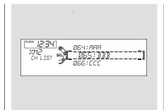
You can also select a channel or category from the list by using the selector knob. Push the selector knob (ENTER) to switch the display to the list displayed with three segments, then turn the knob to select a channel or category. Press the selector knob (ENTER) to set your selection.
