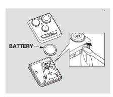
3. Place a cloth on the edge of the keypad to prevent scratches, and remove the upper half by carefully prying on the edge with a small flat-tip screwdriver.
