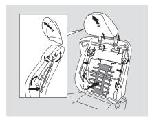
The driver's and front passenger's seats have active head restraints. If the vehicle is struck severely from the rear, the occupant properly secured with the seat belt will be pushed against the seat-back and the head restraint will automatically move forward.
