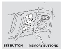
3. Press and release the SET button on the control panel. You will hear a beep. Immediately press and hold one of the memory buttons (1 or 2) until you hear two beeps. The indicator in the memory button will come on. The current position of the driver's seat is now stored.
