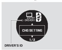
You can customize some vehicle control settings. To enter the customizing mode, press and hold either INFO button (▲/▼) for more than 3 seconds. To change the settings, the ignition switch must be in the ON (II) position, and the vehicle must be stopped with the transmission in Park (automatic) or with the parking brake set (manual).
