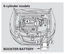
4. Connect one jumper cable to the positive (+) terminal on your battery. Connect the other end to the positive (+) terminal on the booster battery.
