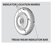
Replace the tire when you can see the tread wear indicator bars. The replacement should be the same size and design tire, mounted on the same wheel. The spare tire is not designed to be mounted on a regular wheel, and the spare wheel is not designed for mounting a regular tire. If you have a flat tire while driving, stop in a safe place to change it. Drive slowly along the shoulder until you get to an exit or an area that is far away from the traffic lanes.
