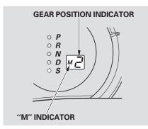
When you move the shift lever from "D" to "S" position and pull either paddle shifter, the gear position indicator displays "M" along with the selected gear number.
