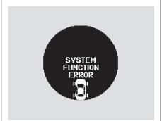
If there is a problem with the TPMS, the tire pressure monitor shows a "SYSTEM FUNCTION ERROR" message and the tire pressure readings are not displayed. If this happens, vou will first see a system warning message "CHECK TPMS SYSTEM" on the multi-information display.
