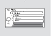
You can also select a file from any of the iPod menus: playlists, artists, albums and songs, by using the interface dial. Press the AUDIO button to display the audio control display on the navigation screen. Push up the interface selector to display the iPod menu. Turn the knob on the interface dial to select a desired list.
