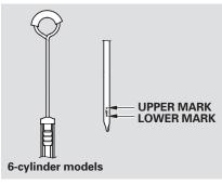
4. Remove the dipstick and check the fluid level. It should be between the upper and lower marks.  If the level is below the lower mark, add fluid into the dipstick hole to bring it to the level between the upper and lower marks.
