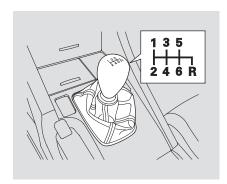
On models with manual transmission. The manual transmission is synchronized in all forward gears for smooth operation. It has a lockout so you cannot accidentally shift from any forward gear to reverse while the vehicle is moving at a certain speed (see page 372).
