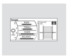
You can also adjust the sound by pushing the \( \)/ \( \)/ (Sound) button repeatedly. Each mode is shown in the center display as it changes. Turn the VOL/ \( \)\( \)\( \) knob to adjust the setting to your liking. When the level reaches the center, you will see "C" in the display.
