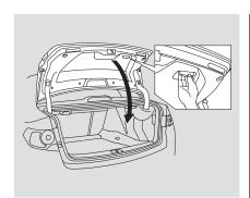
To close the trunk, use the inner handle to lower the lid, then press down on the back edge.
