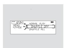
**SHUFFLE OFF** — This feature turns off either of the shuffle modes (SHUFFLE ALL and SHUFFLE ALBUM).
