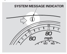
If there is a problem with your vehicle, for example the engine oil level is low or a door is not fully closed, the multi-information display will show you the problem. It does this by interrupting the current display with one or more messages.
