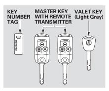
The master key fits all the locks on your vehicle. The valet key works only in the ignition and the driver's door lock. You can keep the glove box locked when you leave your vehicle and the valet key at a parking facility.
