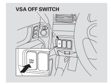
This switch is under the driver's side vent. To turn the VSA system on and off, press and hold it until you hear a beep.
