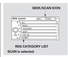
To activate RDS program scan with the interface dial, push the AUDIO button to display the FM radio information on the screen. Push the selector down, and turn the knob to select RDS SEARCH icon. Press ENTER on the selector. The screen shows you the RDS category list.
