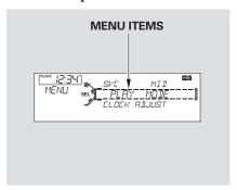
You can select any type of repeat and shuffle mode by using the MENU button and the selector knob. Press the MENU button to display the menu items, then turn the selector knob to select "PLAY MODE." Press ENTER to set the selection.
