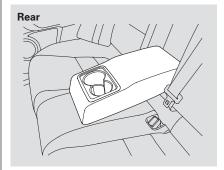
The rear seat armrest is in the center of the rear seat. Pivot it down to use it.
