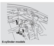
5. Remove the bulb by turning it approximately one-quarter turn counterclockwise.
