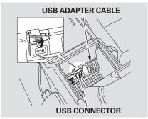
1. Unclip the USB connector by pivoting it, and pull out the USB adapter cable in the console compartment.
