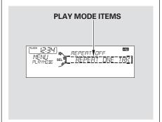
Turn the selector knob to select a play mode: normal play, shuffle off, shuffle all, shuffle album, repeat off, or repeat one track, then press ENTER to set your selection. To cancel the selected mode, press the MENU button and turn the selector knob to show "PLAY MODE," then press ENTER. When you see "NORMAL PLAY," press ENTER again.
