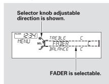
Press the MENU button to display the sound settings. Turn the selector knob to select an appropriate setting: bass, treble, fader, balance, SUBW (subwoofer), SVC (speed-sensitive volume compensation), and CLOCK ADJUST (clock adjustment). Press the selector knob (ENTER) to enter the setting, then turn the selector knob to adjust the setting.
