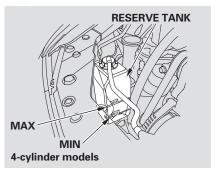
Look at the coolant level in the radiator reserve tank. Make sure it is between the MAX and MIN lines. If it is below the MIN line, see **Adding Engine Coolant** on page 420 for information on adding the proper coolant.
