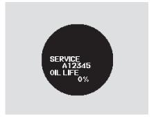
Press the SEL/RESET button on the steering wheel repeatedly to select the engine oil life. The message "SERVICE," along with "0%," and the maintenance item code are displayed on the multi-information display when the calculated engine oil life is 0-1 percent.
