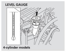
Check the reservoir's fluid level by removing the cap and looking at the level gauge attached to the cap.
