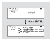
You can also select a file from any list on the iPod menu: playlists, artists, albums and songs, by using the selector knob. Push the selector knob (ENTER) to switch the display to an iPod menu, then turn the selector knob to select a desired list. Press ENTER to set your selection.
