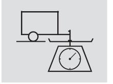
Tongue Load: The weight that the tongue of a fully-loaded trailer puts on the hitch should be approximately 10% of the total trailer weight. Too much tongue load reduces front-tire traction and steering control. Too little tongue load can make the trailer unstable and cause it to sway.
