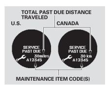
If the indicated required service is not done and the remaining engine oil life becomes 0%, the multi-information display will show a "SERVICE PAST DUE" message, the total distance traveled after the remaining oil life became 0%, and the maintenance item code(s).
