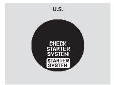
If there is a problem with the starting system, you will see a "CHECK STARTING SYSTEM" message on the multi-information display when the ignition switch is turned to the ON (II) position. You will also see this message when the auto control mode of the starting system has a problem.
