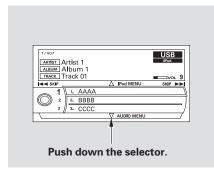
You can select any type of repeat and random mode on the audio menu. Press the AUDIO button to display the audio control screen, then push down the selector to display the audio menu. Turn the knob on the interface dial to select an audio mode: repeat, album random, and track random. Press ENTER to set your selection.
