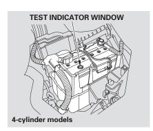
Check the condition of the battery monthly by looking at the test indicator window. The label on the battery explains the test indicator's colors.
