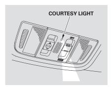
The courtesy light between the spotlights comes on when you turn the parking lights on. To adjust its brightness, turn the instrument panel brightness control knob on the dashboard, with the ignition switch in the ON (II) position (see page 115).
