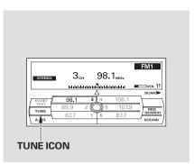
TUNE — Use the TUNE bar to tune the radio to a desired frequency. Press the right side of the bar to tune to a higher frequency, or the left side to tune to a lower frequency. To tune with the interface dial, push the selector down, and turn the knob to TUNE icon. Then press ENTER on the selector, and turn the knob to the desired frequency. To exit the TUNE mode, press ENTER on the selector, then push the selector up.
