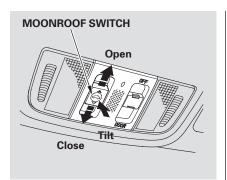
The moonroof can be tilted up in the back for ventilation, or it can be slid back into the roof. Use the switch on the front ceiling to operate the moonroof. You must turn the ignition switch to the ON (II) position to operate the moonroof.
