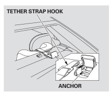
6. Route the tether strap through the legs of the head restraint and over the seat-back, making sure the strap is not twisted.
