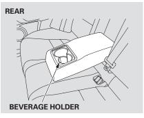
The rear seat also has a beverage holder in the center armrest. To use it, pivot the armrest down.
