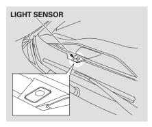
The automatic lighting feature is controlled by a sensor located on top of the dashboard. Do not cover this sensor or spill liquids on it. Automatic Lighting Off Feature
