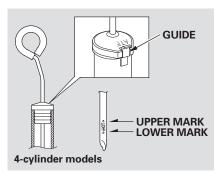
3. Insert the dipstick all the way back into the transmission securely as shown in the illustration.
