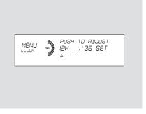
4. Turn the selector knob to select the item which you want to adjust. Turning the selector knob will change the selected item between the clock display setting, hours, minutes, and SET. The selected item is indicated with △ in the display.
