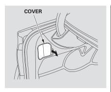
If there is a problem with the power door lock system and you cannot unlock the driver's door, use the release lever behind the left side cover in the trunk.
