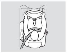
If you ever have a moderate to severe side impact, sensors will detect rapid acceleration and signal the control unit to instantly inflate either the driver's or the passenger's side airbag.
