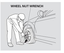
7. Loosen each wheel nut 1/2 turn with the wheel nut wrench.
