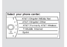
**NOTE:** For the Phone Data Connection button to be active, you need a *Bluetooth*® compatible and enabled cell phone paired to the *Bluetooth*® HandsFreeLink® (HFL). To complete the data connection setup, the paired phone must have a compatible data service.
