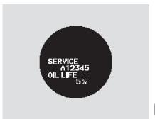
Press the SEL/RESET button on the steering wheel repeatedly to select the engine oil life. The message "SERVICE," along with "5%," and the maintenance item code are displayed on the multi-information display when the calculated engine oil life is 1–5 percent (see page 403).
