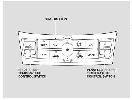
To set the driver's side temperature to a different value than the passenger's, press the DUAL button, then push the switch up or down on the driver's side. To set the passenger's side to a different value than the driver's, push the switch up or down on the passenger's side. You can adjust the passenger's side without pressing the DUAL button first.
