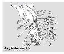
To access the radiator reserve tank, remove the right-side engine compartment cover.
