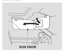
To use the sun visor, pull it down. You can also use the sun visor at the side window. Remove the support rod from the clip and swing the sun visor toward the side window.
