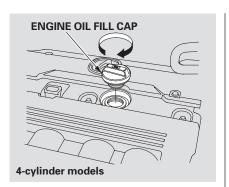
Unscrew and remove the engine oil fill cap on top of the valve cover. Pour in the oil slowly and carefully so you do not spill any. Clean up any spills immediately. Spilled oil could damage components in the engine compartment.
