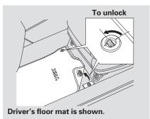
The driver's floor mat that came with your vehicle hooks over the floor mat anchors. To lock each anchor, turn the knob clockwise. This keeps the floor mat from sliding forward and possibly interfering with the pedals.
