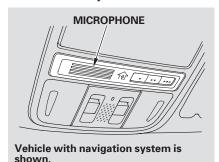
• Air or wind noise from the dashboard and side vents, windows and moonroof may interfere with the microphone. Adjust or close them as necessary.
