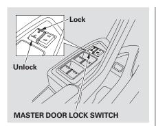
To lock all doors, push the front of the master door lock switch on either front door, pull the lock tab rearward on the driver's door, or use the key on the outside lock on the driver's door.
