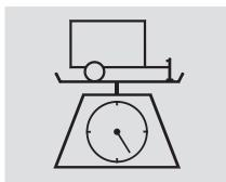
Total Trailer Weight: The maximum allowable weight of the trailer and everything in or on it must not exceed 1,000 lbs (450 kg). Towing a load that is too heavy can seriously affect your vehicle's handling and performance. It can also damage the engine and drivetrain.
