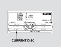
To select a different disc, press the corresponding number on the preset buttons, or turn the interface knob to highlight the desired disc number, then press ENTER on the interface selector.
