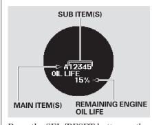
Press the SEL/RESET button on the steering wheel repeatedly to select the engine oil life information. Along with the "OIL LIFE" message, you will see the percentage of the remaining engine oil life and the maintenance item codes on the multi-information display.
