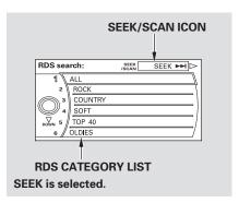
To activate RDS program search with the interface dial, push the AUDIO button to display the FM radio information on the screen. Push the selector down, and turn the knob to select RDS SEARCH icon. Press ENTER on the selector. The screen shows you the RDS category list.
