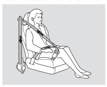
For added protection, the front seat belts are equipped with automatic seat belt tensioners. When activated, the tensioners immediately tighten the belts to help hold the driver and a front passenger in position. The tensioners are designed to activate in any collision severe enough to cause the front airbags to deploy.
