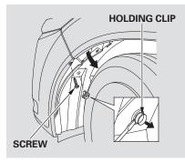
2. Use a flat-tip screwdriver to remove the holding clip from the inner fender, and remove the screw with a Phillips-head screwdriver.
