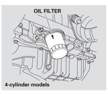
5. Remove the oil filter and let the remaining oil drain. A special wrench (available from your dealer) is required.
