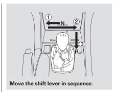
1. With the clutch pedal pressed, move the shift lever to the first/second gear side of the neutral gate, then shift to reverse.
