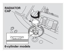
4. Remove the radiator cap by pushing down and turning counterclockwise.
