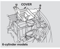
6-cylinder models Remove the fasteners, then remove the air intake duct cover.
