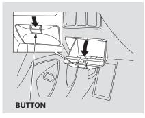
To open the driver's pocket, push the button on the lid. To close it, push the lid up until it latches.
