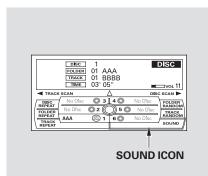
To adjust them, press the AUDIO button, push the interface selector down, and turn the interface knob to SOUND. Then press ENTER on the selector.
