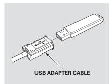
2. Connect the USB flash memory device to the USB adapter cable correctly and securely.
