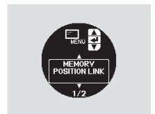
If "MEMORY POSITION LINK" is set to "ON," the driver's seat moves to the position stored in the memory (see page 142) when you open the driver's door, using the remote transmitter.
