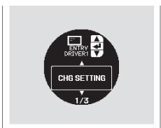
When you want to change the vehicle control settings, press the INFO (▲/▼) button to select CHG SETTING, then press the SEL/RESET button.
