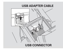
Unclip the USB connector by pivoting it, and pull out the USB adapter cable in the console compartment.
