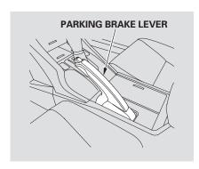
To apply the parking brake, pull the lever up fully. To release it, pull up slightly, push the button, and lower the lever. The parking brake indicator on the instrument panel should go out when the parking brake is fully released (see page 61).
