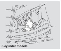
6. Install a new oil filter according to the instructions that come with it. Make sure to clean off any dirt and dust on the contacting surface of a new oil filter.
