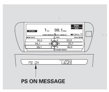
To switch the PS name display function on and off, press and release the TITLE button. With the system on, you will see the "PS ON" message on the center display. If the station you are listening to is an RDS station, the displayed frequency switches to the station name.
