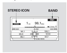
The ignition switch must be in the ACCESSORY (I) or the ON (II) position. Press the AUDIO button to view the audio control display. Turn the system on by pressing the VOL/ (b) knob or the FM/AM button. Adjust the volume by turning the VOL/ (b) knob.
