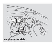
4. Remove the electrical connector from the bulb by pushing on the tab to unlock it, then slide the connector off the bulb.
