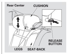
Removing the Head Restraint
