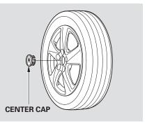
15.Remove the center cap before storing the flat tire in the trunk well.
