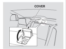
2. Pull up the cover of the tether anchor point on the left side.
