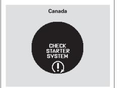
If this message is on, the ignition switch has to be held in the START (III) position manually until the engine starts. The ignition switch can be held in that position up to 15 seconds.
