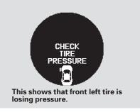
Each tire has its own pressure sensor. If the air pressure of a tire becomes significantly low, the sensor in that tire immediately sends a signal that causes the low tire pressure/TPMS indicator in the instrument panel to come on. If this happens, you will see which tire is losing pressure on the multi-information display along with a "CHECK TIRE PRESSURE" message.
