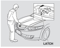
2. Reach in between the hood and the front grille with your fingers. The hood latch handle is above the "A" logo. Push this handle up to the right until it releases the hood. Lift the hood.
