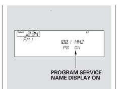
To switch the function between on and off, press and release the TITLE button. With the system on, you will see the "PS ON" message on the display. If the station you are listening to is an RDS station, the displayed frequency switches to the station name.
