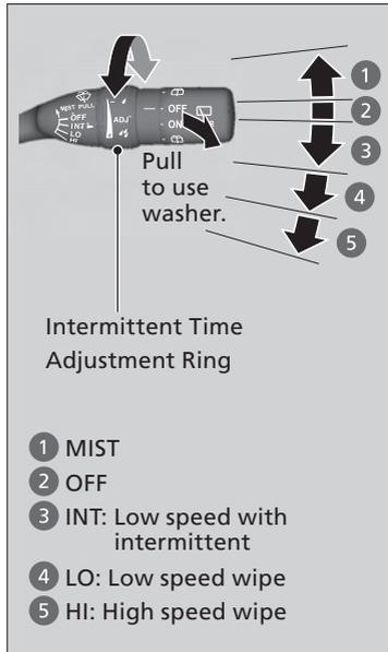
The windshield wipers and washers can be used when the ignition switch is in ON **II**.
