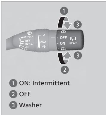
The rear wiper and washer can be used when the ignition switch is in ON .
