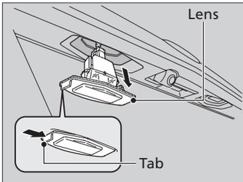
1. Push the tab on the left and pull out the lens and the socket attached to it.
