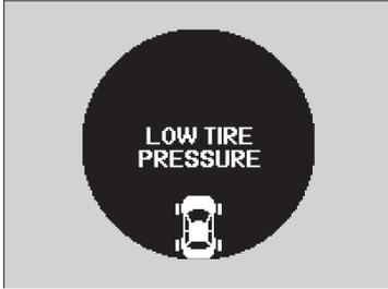
If any tire has low pressure, "LOW TIRE PRESSURE" is displayed on the multi-information display. Check the pressure of each tire by pressing the SEL/RESET button.
