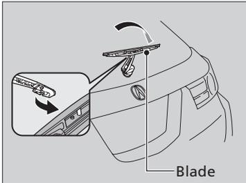
2. Pivot up the bottom end of the wiper blade until it comes off from the wiper arm.
