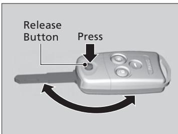
Use the keys to start and stop the engine, and to lock and unlock all the doors, tailgate, and fuel fill door. You can also use the remote transmitter to lock and unlock the doors, tailgate, and fuel fill door.
