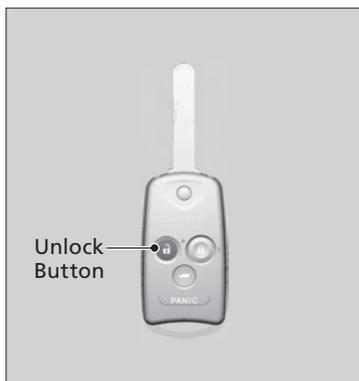
**To open:** Press the UNLOCK button twice within 10 seconds and hold it down for the second time. If the windows stop midway, repeat the procedure.
