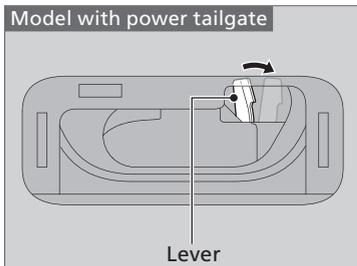
2. To open the tailgate, pull the tailgate while pushing down the lever.
