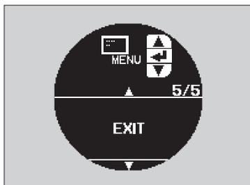
4. Press the /▼ button until "TRIP A RESET with REFUEL" appears on the display, then press the SEL/RESET button.
