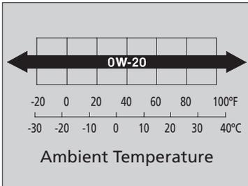
Use Genuine Acura Motor Oil or another commercial engine oil of suitable viscosity for the ambient temperature as shown below.
