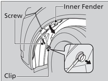
1. Turn the steering wheel all the way to the opposite side from the headlight being replaced.
