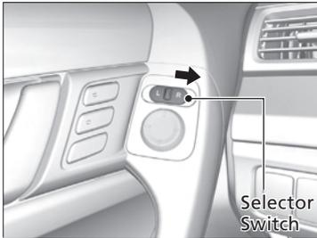
If activated, the passenger side door mirror automatically tilts downward when you put the shift lever in **R**; this improves close-in visibility on the passenger side of the vehicle when backing up. The mirror automatically returns to its original position when you shift out of **R**.
