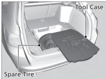
3. Take the tool case out of the cargo. Take the jack and wheel nut wrench out of the tool case.
