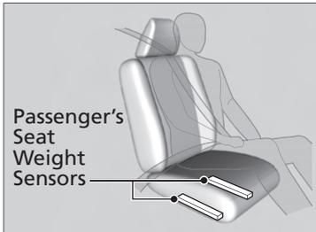
The passenger's advanced front airbag system includes weight sensors.
