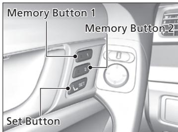
1. Adjust the driver's seat to the desired position, and turn the ignition switch to ON **II**.
