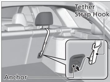
3. Release the head restraint, then route the tether strap between the head restraint legs, and secure the tether strap hook onto the anchor.
