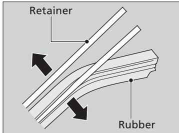
4. Remove the retainer from wiper blade and mount it to a new rubber blade.
