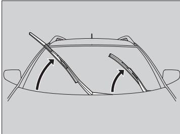
1. Lift the driver side wiper arms first, then the passenger side.
