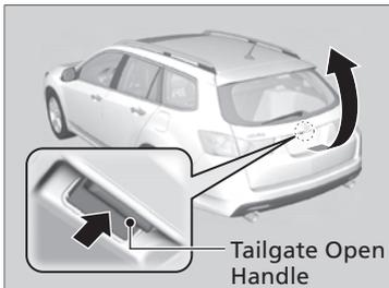
When all the doors are unlocked, the tailgate is unlocked. Push the tailgate open handle and lift open the tailgate.
