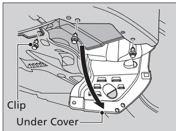
1. Remove the clip using a flat-tip screwdriver, and lower the under cover.
