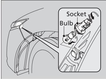
3. Turn the socket to the left and remove it.
