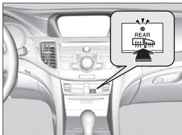
Press the rear defogger and heated door mirror button to defog the rear window and mirrors when the ignition is in ON
