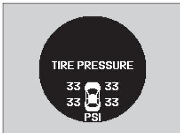
To display the pressure of all four tires, press the SEL/RESET button.
