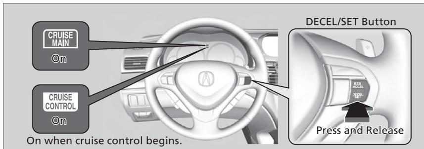
Press the DECEL/SET button when you reach the desired speed using the accelerator pedal.
