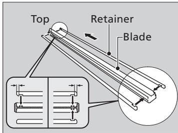
5. Remove the retainer from the rubber blade that has been removed, and mount to a new rubber blade.
