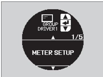
2. Press the SEL/RESET button to go into the "METER SETUP" group.
