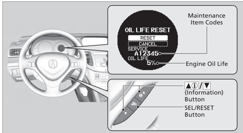
1. Turn the ignition switch to ON
