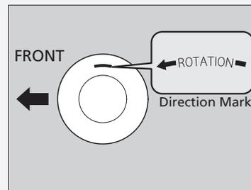
When the tires are rotated, make sure the air pressures are checked.
