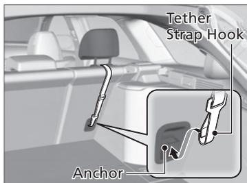
■ **Using an outer anchor**
