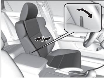
The firmness of the seat-back can be adjusted.
