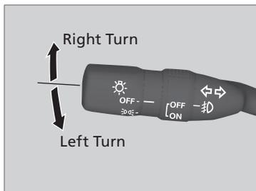
The turn signals can be used when the ignition switch is in ON
