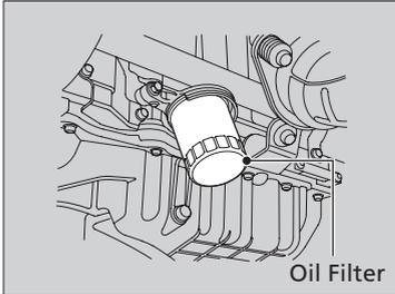
6. Check that the filter gasket is not stuck to the engine contact surface.
