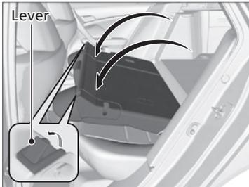
2. Pull the release lever and fold down the seat-back.
