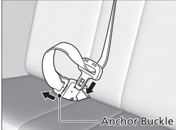
1. Unlatch the detachable anchor from the anchor buckle and store the detachable anchor in the retractor housing.
