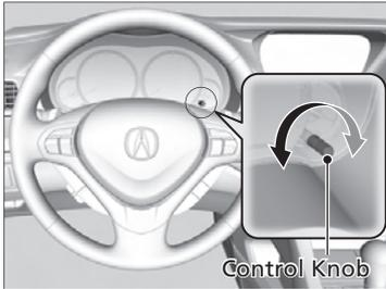
When the parking lights are turned on and the ignition switch is in ON
