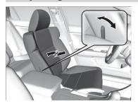
The firmness of the seat-back can be adjusted.
