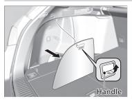
Located on the side panel in the cargo area. Pull up the handle and remove the lid.
