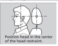
Your vehicle is equipped with head restraints.
