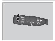
Automatic lighting control can be used when the ignition switch is in ON  $\boxed{II}$ .
