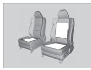
If the ignition switch is in ON II. The HI setting heats the seats faster than the LO setting.
