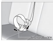
**1.** Unlatch the detachable anchor from the anchor buckle and store the detachable anchor in the retractor housing.
