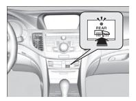
Press the rear defogger and heated door mirror button to defog the rear window and mirrors when the ignition is in ON  $\boxed{\rm II}$ .
