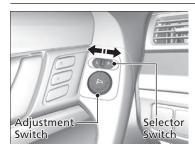
You can adjust the door mirrors when the ignition switch is in ON []].
