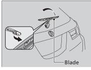
Pivot up the bottom end of the wiper blade until it comes off from the wiper arm. ○ Changing the Rear Wiper Blade Rubber
