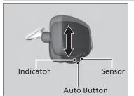
When driving after dark, the automatic dimming rearview mirror reduces the glare from headlights behind you. Press the AUTO button to turn this function on and off. When activated, the AUTO indicator comes on.
