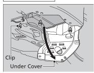
**1.** Remove the clip using a flat-tip screwdriver, and lower the under cover.
