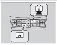
Pressing the button turns the air conditioner system on and automatically switches the system to fresh air mode.
