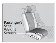
The passenger's advanced front airbag system includes weight sensors.
