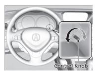
When the parking lights are turned on and the ignition switch is in ON [II], you can use the brightness control knob to adjust instrument panel brightness.
