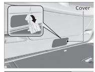
**1.** Use a flat-tip screwdriver and remove the cover on the back of the tailgate.
