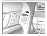
If activated, the passenger side door mirror automatically tilts downward when you put the shift lever in  $\boxed{R}$ ; this improves close-in visibility on the passenger side of the vehicle when backing up. The mirror automatically returns to its original position when you shift out of  $\boxed{R}$ .
