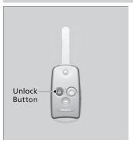
**To open:** Press the UNLOCK button twice within 10 seconds and hold it down for the second time. If the windows stop midway, repeat the procedure.
