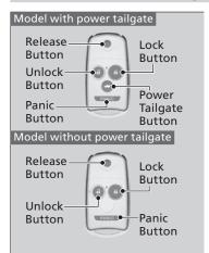
Use the keys to start and stop the engine, and to lock and unlock all the doors, tailgate, and fuel fill door. You can also use the remote transmitter to lock and unlock the doors, tailgate, and fuel fill door.
