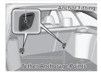
Two tether anchorage points are provided behind the rear outer seating positions and one in the ceiling for the rear center. A child seat that is installed with a seat belt and comes with a tether can use the tether for additional security.
