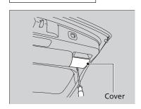
**1.** Remove the cover by prying on the edge of the cover using a flat-tip screwdriver.
