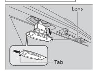
**1.** Push the tab on the left and pull out the lens and the socket attached to it.
