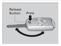
The master key folds up inside the remote transmitter.
