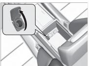
There are three accessory power sockets; one in the console compartment, one in the front of the center console, and one in the left side panel in the cargo area. They can be used when the ignition switch is in ACCESSORY I or ON II.
