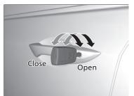
**To open:** Unlock the driver's door with the key. Within 10 seconds of returning the key to the central position, turn the key in the unlock direction and hold it there.
