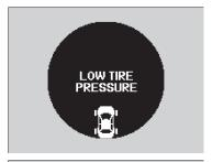
If any tire has low pressure, "LOW TIRE PRESSURE" is displayed on the multi-information display. Check the pressure of each tire by pressing the SEL/RESET button.
