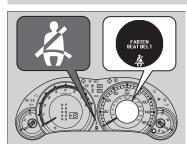
Your vehicle monitors front seat belt use. If the ignition switch is turned to ON III before the driver's seat belt is fastened, a beeper will sound and the indicator will blink. If the driver does not fasten the belt before the beeper stops, the indicator will remain on.
