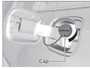
**5.** Remove the fuel fill cap slowly. If you hear a release of air, wait until this stops, then turn the knob slowly to open the fuel fill cap.
