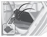
**2.** Pull the release lever and fold down the seat-back.
