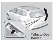
When all the doors are unlocked, the tailgate is unlocked. Push the tailgate open handle and lift open the tailgate.
