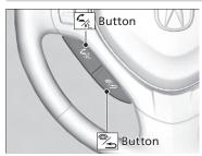
Press the  $\bigcirc$  (HFL Talk) button on the steering wheel to receive a call when  $Bluetooth^{®}$  Audio is playing.
