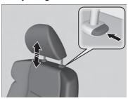
**To raise the head restraint:** Pull it upward. **To lower the head restraint:** Push it down while pressing the release button.
