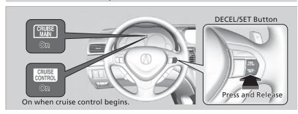
Press the DECEL/SET button when you reach the desired speed using the accelerator pedal.
