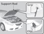
Remove the support rod from the clamp using the grip. Mount the support rod in the hood.
