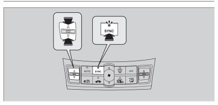
You can set the temperature synchronously for the driver side and the passenger side in synchronized mode.
