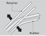
**4.** Remove the retainer from wiper blade and mount it to a new rubber blade.
