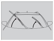
**1.** Lift the driver side wiper arms first, then the passenger side.
