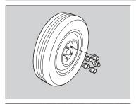
1. Remove the wheel nuts and flat tire.
