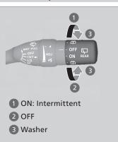
The rear wiper and washer can be used when the ignition switch is in ON  $\boxed{\rm II}$ .
