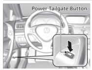
To open or close the power tailgate, press the tailgate button in the driver's door for about one second. The beeper sounds and some exterior lights flash.
