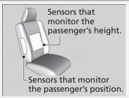
The sensors that monitor the front passenger's height and body position may not work if:
