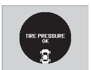
To select the tire pressure monitor, turn the ignition switch to ON II and press the ▲③/▼ (information) button until you see the tire pressure screen.
