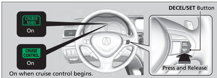
Press the **DECEL/SET** button when you reach the desired speed using the accelerator pedal.
