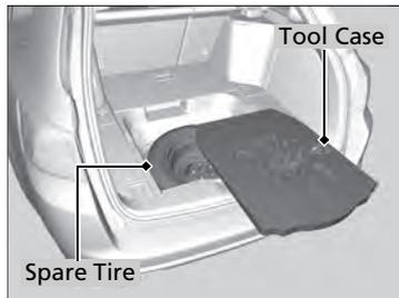
3. Take the tool case out of the cargo area. Take the jack and wheel nut wrench out of the tool case.
