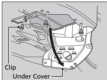
1. Remove the clips using a flat-tip screwdriver, and lower the under cover.
