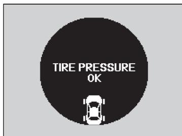
To select the tire pressure monitor, turn the ignition switch to ON **II** and press the **▲①/▼** (information) button until you see the tire pressure screen.
