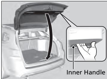
To manually close the tailgate, grab the inner handle, pull the tailgate down, and push it closed from the outside.
