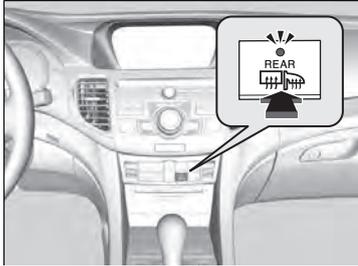
Press the rear defogger and heated door mirror button to defog the rear window and mirrors when the ignition is in ON
