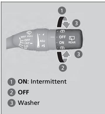
The rear wiper and washer can be used when the ignition switch is in ON
