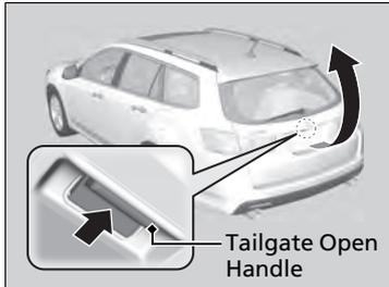
When all the doors are unlocked, the tailgate is unlocked. Pull the tailgate open handle and lift open the tailgate.
