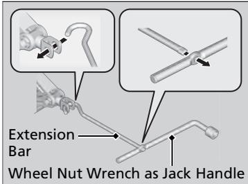
3. Raise the vehicle, using the extension bar and the jack handle, until the tire is off the ground.
