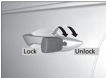
Fully insert the key and turn it. If you are using the master key, make sure it is fully extended.
