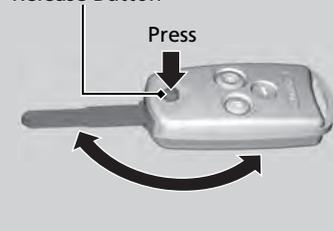
Use the keys to start and stop the engine, and to lock and unlock all the doors, tailgate, and fuel fill door. You can also use the remote transmitter to lock and unlock the doors, tailgate, and fuel fill door.
