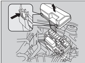
Located near the brake fluid reservoir. Push the tabs to open the box.
