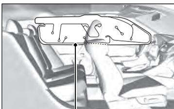
Deployed Side Curtain Airbag
