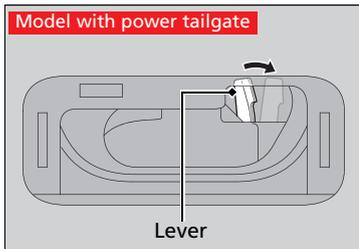
2. To open the tailgate, pull the tailgate while pushing down the lever.
