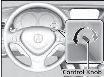
When the parking lights are turned on and the ignition switch is in ON
