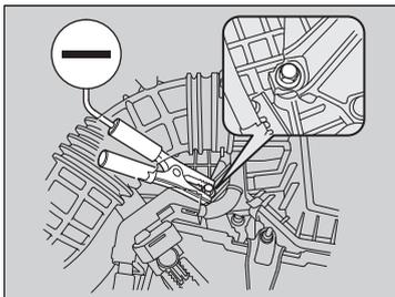
3. Connect the second jumper cable to the assisting vehicle's  $\ominus$  terminal.
