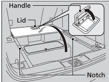
Lift up the handle and put the lid on the notch.
