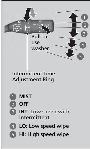
The windshield wipers and washers can be used when the ignition switch is in ON
