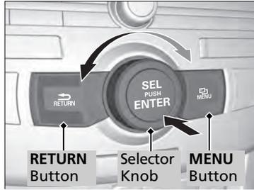
Press the **MENU** button, and rotate
