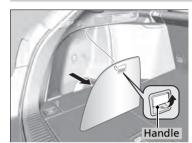
Located on the side panel in the cargo area. Pull up the handle and remove the lid.
