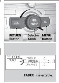
Press the **MENU** button, and rotate  $^{\circ}$  to adjust the setting. Rotate  $^{\circ}$  to scroll through the following choices:
