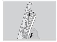
► Make sure it is engaged correctly, then install the wiper blade assembly onto the wiper arm.
