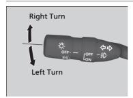
The turn signals can be used when the ignition switch is in ON  $\overline{\text{II}}$ .
