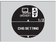
1. Press and hold the ▲①/▼ button until CHG SETTING appears on the display.
