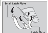
**1.** Pull out the seat belt's small latch plate and the latch plate from each holding slot in the ceiling.
