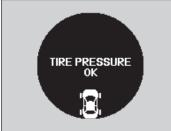
To select the tire pressure monitor, turn the ignition switch to ON III and press the (information) button until you see the tire pressure screen.
