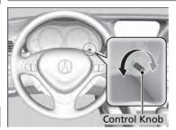
When the parking lights are turned on and the ignition switch is in ON  $\boxed{II}$ , you can use the brightness control knob to adjust instrument panel brightness.
