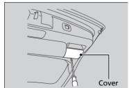
**1.** Remove the cover by prying on the edge of the cover using a flat-tip screwdriver.
