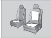
The ignition switch must be in ON III to use the seat heaters. The **HI** setting heats the seats faster than the **LO** setting.
