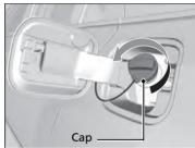
**5.** Remove the fuel fill cap slowly. If you hear a release of air, wait until this stops, then turn the knob slowly to open the fuel fill cap.
