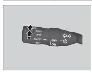
Automatic lighting control can be used when the ignition switch is in ON [II].
