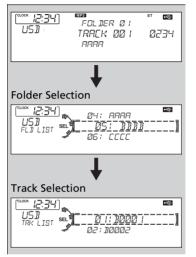
**1.** Press  $\overline{\&}$  to switch the display to a folder list.
