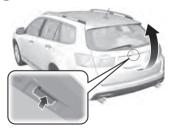
With all the doors unlocked, pull the tailgate open handle on the tailgate to open it.
