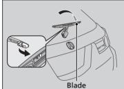
**2.** Pivot up the bottom end of the wiper blade until it comes off from the wiper arm.
