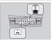
Pressing the button turns the air conditioner system on and automatically switches the system to fresh air mode.
