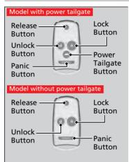
Use the keys to start and stop the engine, and to lock and unlock all the doors, tailgate, and fuel fill door. You can also use the remote transmitter to lock and unlock the doors, tailgate, and fuel fill door.
