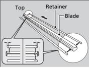
**5.** Remove the retainers from the rubber blade that has been removed, and mount to a new rubber blade.
