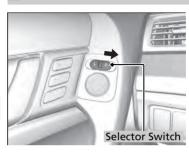
If activated, the passenger side door mirror automatically tilts downward when you put the shift lever in R; this improves close-in visibility on the passenger side of the vehicle when backing up. The mirror automatically returns to its original position when you shift out of R.
