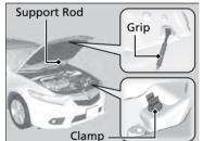
**4.** Remove the support rod from the clamp using the grip. Mount the support rod in the hood.
