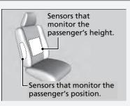
The sensors that monitor the front passenger's height and body position may not work if:
