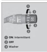
The rear wiper and washer can be used when the ignition switch is in ON  $\boxed{II}$ .
