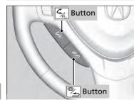
Press the (HFL Talk) button on the steering wheel to receive a call when *Bluetooth* Audio is playing.
