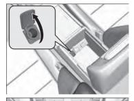
There are three accessory power sockets; one in the console compartment, one in the front of the center console, and one in the left side panel in the cargo area. They can be used when the ignition switch is in ACCESSORY I or ON III.
