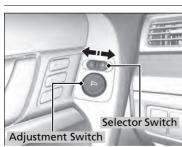
You can adjust the door mirrors when the ignition switch is in ON [II].
