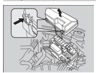
Located near the brake fluid reservoir. Push the tabs to open the box.
