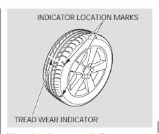
Your tires have wear indicators molded into the tread. When the tread wears down, you will see a band 1/2 inch (12.7 mm) wide across the tread. This shows there is less than 1/16 inch (1.6 mm) of tread left on the tire
