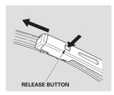
2. Disconnect the blade assembly from the wiper arm by pushing in the release button. Then slide the blade assembly out of the wiper arm.
