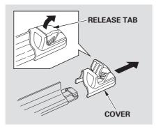
3. Pull up the cover release tab on the end of the blade assembly, then remove the cover.
