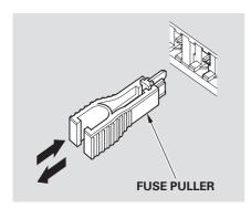
4. Check the smaller fuses in the under-hood fuse boxes and all the fuses in the interior fuse box by pulling out each one with the fuse puller provided in the primary under-hood fuse box.
