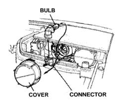
3. Remove the cover from the back of the burned-out bulb by turning it counterclockwise.
