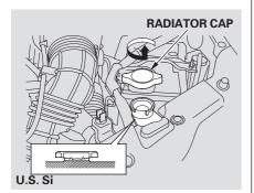
3. Remove the radiator cap by pushing down and turning counterclockwise.
