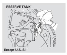
4. The coolant level should be up to the base of the filler neck. Add coolant if it is low.
