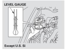
Check the fluid level by removing the cap and looking at the level gauge.
