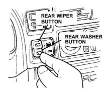
The rear window wiper cannot be operated when the rear window is not latched.
