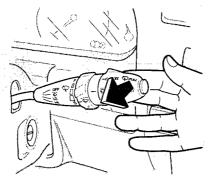
To operate the windshield washers, pull back on the windshield wiper control lever. The washers will spray, and the wipers will run at low speed, for as long as you hold the lever. The wipers will continue to run for a short time after you release the lever.
