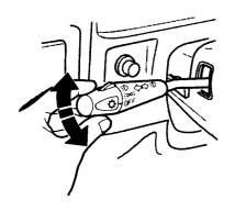
The turn signal will cancel itself as the turn is completed. In some driving maneuvers, such as changing lanes on an expressway, the steering wheel is not turned back sufficiently after completing the turn to automatically cancel the turn signal. In such maneuvers the driver should manually return the lever to the neutral or canceled position when the turn is completed.
