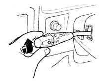
The rotating switch on the left lever controls the lights. Rotating this switch to the DOT position turns on the instrument panel lights and all exterior lights except the headlights. Rotating the switch to the Dosition turns on the headlights.
