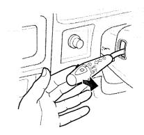
To flash the high beams, pull the lever back about half way and then let it go. The high beams will stay on for as long as you hold the lever back, no matter what position the headlight switch is in.
