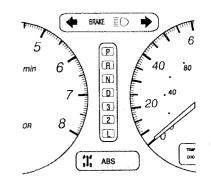
The shift lever position indicator is in the instrument panel. The appropriate letter or number illuminates to show what position the shift lever is in.
