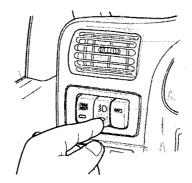
When fog or heavy mist reduces your forward vision, push this switch to turn the fog lights on. The indicator light in the switch turns on. Push the switch again to turn off the fog lights.
