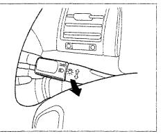
To change between low beams and high beams, pull the turn signal lever until you hear a click, then let go. The blue high beam indicator will light (see page 33). To flash the high beams, pull the turn signal lever back lightly, then release it. The high beams will come on and go off.
