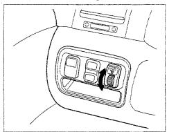
The dial on the dashboard to the left of the instrument panel controls the brightness of the instrument panel lights. Turn the dial to adjust the brightness.
