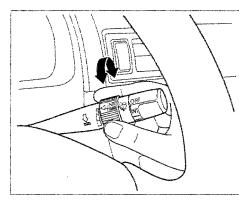
In intermittent, the wipers operate every few seconds. You can vary how often the wipers sweep the windshield by turning the INT TIME ring next to the rotary switch. In low speed and high speed, the wipers run continuously.
