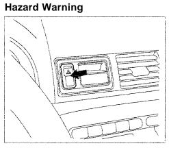
Push the red button to the left of the clock to turn on the hazard warning lights (four-way flashers). This causes all four outside turn signals and both indicators in the instrument panel to flash. Use the hazard warning lights if you need to park in a dangerous area near heavy traffic, or if your car is disabled.
