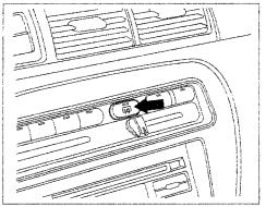
The rear window defogger will clear fog, frost, and thin ice from the window. Push the defogger button to turn it on and off. The light in the button lights to show the defogger is on. If you do not turn it off, the defogger will shut itself off after about 25 minutes. It also shuts off when you turn off the ignition. You have to turn it on again when you restart the car.
