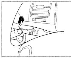
The rotating switch on the left lever controls the lights. Turning this switch to the " ₹D0€" position turns on the parking lights, taillights, instrument panel lights, side-marker lights, and rear license plate lights. Turning the switch to the " ≣D" position turns on the headlights. If you leave the lights on with the ignition switch in ACCESSORY (I) or LOCK (0), you will hear a reminder chime when you open the driver's door.
