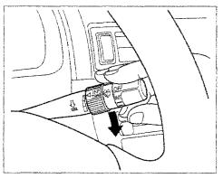
To operate the wipers in mist mode, push the control lever down. The wipers run at high speed until you release the lever. This gives you a quick way to clear the windshield.
