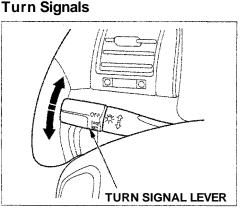
Signal a turn or lane change with this lever. Push down on the lever to signal a left turn, and up to signal a right turn. If you push it up or down all the way, the turn signal continues to blink even when you release the lever. It shuts off automatically as you complete the turn. To signal a lane change, push lightly on the turn signal lever in the proper direction and hold it. The lever will return to the center position as soon as you release it.
