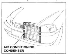
Periodically check the engine's radiator and air conditioning condenser for leaves, insects, and dirt stuck to the front surface. These block the air flow and reduce cooling efficiency. Use a light spray from a hose or a soft brush to remove them.
