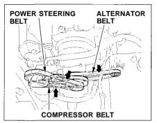
Check the condition of the two or three drive belts. Examine the edges of each belt for cracks or fraying. Check the tension of each belt by pushing on it with your thumb midway between the pulleys. The belts should have the following "play" or deflection. Alternator belt: 8.0-10.5 mm (0.31-0.41 in)Power steering belt: 10.5-14.0 mm (0.41-0.55 in)
