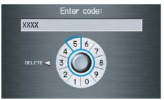
Enter the four-digit security code. If you have entered it correctly, the display changes to the **Disclaimer** screen. If you make a mistake, the system will display "INCORRECT PIN." Re-enter your 4-digit security code.
