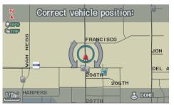
4. Rotate the **Interface Dial knob** so the vehicle position arrowhead is pointing in the correct direction, and push in on the **Interface Dial**. The display will return to the previous screen.
