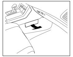
2. Remove the DVD while the ignition switch is in the ACCESSORY (I) position or in the ON (II) position. 3. Push the **OPEN** button. An error message will be displayed on the screen. This is normal.
