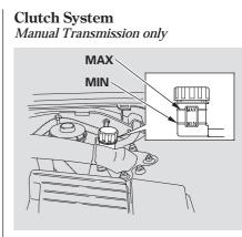
The fluid level should be between the MIN and MAX marks on the side of the reservoir. If it is not, add brake fluid to bring it up to that level. Use the same fluid specified for the brake system.
