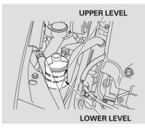
Check the level on the side of the reservoir when the engine is cold, and the engine compartment rightside cover is off (see page 213). The fluid should be between the UPPER LEVEL and LOWER LEVEL. If not, add power steering fluid to the UPPER LEVEL mark. Pour the fluid slowly and carefully so you do not spill. Clean up any spill immediately; it could damage components in the engine compartment.
