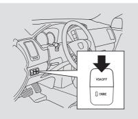
This switch is under the left vent. Press it to turn the vehicle stability assist system on and off.
