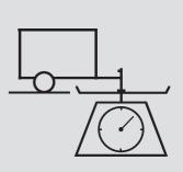
**Gross Vehicle Weight Rating** (GVWR) — The maximum allowable weight of the vehicle, all occupants, all cargo and the tongue load is 5,950 lbs (2,700 kg).
