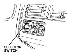
Adjust the outside mirrors with the adjustment switch on the left side of the dashboard:
