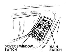
The driver's armrest has a master power window control panel. To open any of the passengers' windows, push down on the appropriate switch and hold it down until the window reaches the desired position. To close the window, push up on the window switch. Release the switch when the window gets to the position you want.
