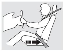
Adjust the driver's seat as far to the rear as possible while allowing you to maintain full control of the vehicle. Have a front passenger adjust their seat as far to the rear as possible. If you sit too close to the steering wheel or dashboard, you can be seriously injured by an inflating front airbag, or by striking the steering wheel or dashboard.
