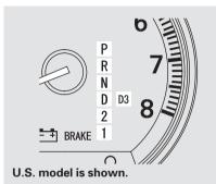
These indicators on the instrument panel show which position the shift lever is in. The "D" indicator comes on for a few seconds when you turn the ignition switch to the ON (II) position. If it flashes while driving (in any shift position), it indicates a possible problem in the transmission.
