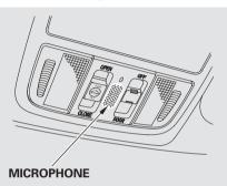
• Air or wind noise from the dashboard and side vents and all windows may interfere with the microphone. Adjust or close them as necessary.
