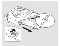
3. To install a CD into the magazine, push the button while pulling out on the tab.
