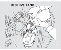
If the coolant level in the reserve tank is at or below the MIN line, add coolant to bring it up to the MAX line. Inspect the cooling system for leaks. Always use Honda Long-life Antifreeze/Coolant Type 2. This coolant is pre-mixed with 50 percent antifreeze and 50 percent distilled water. Never add straight antifreeze or plain water.
