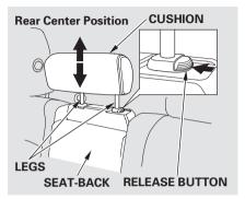
Removing the Head Restraint
