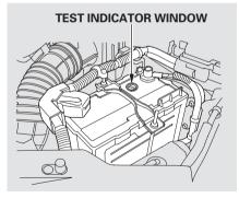
Check the terminals for corrosion (a white or yellowish powder). To remove it, cover the terminals with a solution of baking soda and water. It will bubble up and turn brown. When this stops, wash it off with plain water. Dry off the battery with a cloth or paper towel. Coat the terminals with grease to help prevent future corrosion.
