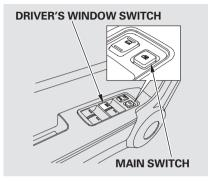
Turn the ignition switch to the ON (II) position to raise or lower any window. To open the window, push the switch down and hold it. Release the switch when you want to stop the window. To close the window, pull back on the switch and hold it.
