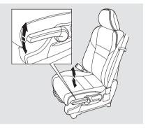
The height of your driver's seat is adjustable. To raise the seat, repeatedly pull up the lever on the outside of the seat cushion. To lower the seat, push the lever down repeatedly.
