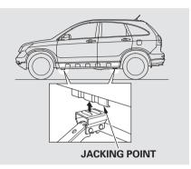
8. Place the jack under the jacking point nearest the tire you need to change. Turn the end bracket clockwise until the top of the jack contacts the jacking point. Make sure the jacking point tab is resting in the jack notch.
