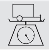
**Total Trailer Weight:** The maximum allowable weight of the trailer and everything in or on it must not exceed 1,500 lbs (680 kg). Towing a load that is too heavy can seriously affect your vehicle's handling and performance. It can also damage the engine and drivetrain.
