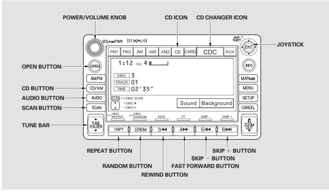
**Loading CDs in the Changer** Your vehicle has the CD changer in the center console.
