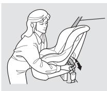
1. With the child seat in the desired seating position, route the belt through the child seat according to the seat maker's instructions. then insert the latch plate into the buckle and remove any slack from the lap portion of the belt.
