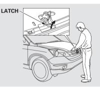
2. Reach in between the hood and the front grille with your fingers. The hood latch handle is above the "H" logo. Push this handle up until it releases the hood. Lift the hood.
