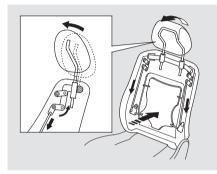
The driver's and front passenger's seats have active head restraints. If the vehicle is struck severely from the rear, the occupant properly secured with the seat belt will be pushed against the seat-back and the head restraint will automatically move forward. This reduces the distance between the restraint and the occupant's head. It also helps protect the occupants against the likelihood of whiplash and injuries to the neck and upper spine.
