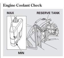
Look at the coolant level in the radiator reserve tank. Make sure it is between the MAX and MIN lines. If it is below the MIN line, see **Adding Engine Coolant** on page 352 for information on adding the proper coolant.
