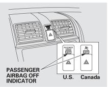
This indicator alerts you that the passenger's front airbag has been shut off because weight sensors detect about 65 lbs (29 kg) or less (the weight of an infant or small child) on the front passenger's seat. It does *not mean* there is a problem with the airbag. Be aware that objects placed on the front seat can cause the indicator to come on.
