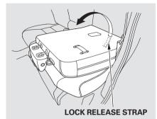
3. Unlock the seat from the floor by pulling the lock release strap located at the rear of the seat cushion, under the seat back, then lift the rear of the seat. You cannot fold up the rear seat if it is not latched securely in the rearmost position.
