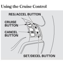
1. Push the CRUISE button on the steering wheel. The CRUISE MAIN indicator on the instrument panel comes on.
