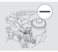
4. Connect the second jumper cable to the negative (-) terminal on the booster battery. Connect the other end to the stud bolt on the engine side as shown. Do not connect this jumper cable to any other part of the engine.
