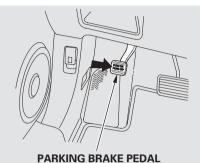
To apply the parking brake, push the pedal down with your foot. To release it, push on the pedal again. The parking brake indicator on the instrument panel should go out when the parking brake is fully released (see page 62).
