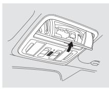
The sunglasses holder uses a convex mirror for its bottom panel. You can see all the vehicle passengers in this mirror. To use the mirror, open the sunglasses holder fully, push it to the first detent, and release it.
