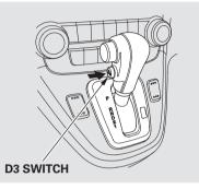
Press the D3 switch on the side of the shift lever to turn this mode on or off; the D3 mode indicator comes on whenever the D3 mode is selected.
