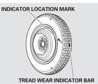
Replace the tire when you can see the tread wear indicator bars. The replacement tire should be the same size and design, mounted on the same wheel. The spare tire is not designed to be mounted on a regular wheel, and the spare wheel is not designed for mounting a regular tire. If you have a flat tire while driving, stop in a safe place to change it. Drive slowly along the shoulder until you get to an exit or an area to stop that is far away from the traffic lanes.
