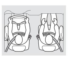
Your vehicle also has side airbags to help protect the upper torso of the driver or a front seat passenger during a moderate to severe side impact (see page 29 for more information on how your side airbags work).
