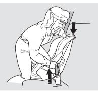
4. After confirming that the belt is locked, grab the shoulder part of the belt near the buckle, and pull up to remove any slack from the lap part of the belt. Remember, if the lap part of the belt is not tight, the child seat will not be secure.
