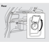
Make sure to put the socket cover back in place to prevent any small foreign objects from getting into the socket.
