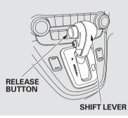
To shift from any position, press firmly on the brake pedal and the release button on the side of the shift lever. You cannot shift out of Park when the ignition switch is in the LOCK (0) or ACCESSORY (I) position.
