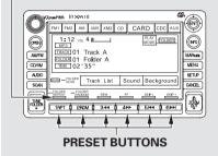
You can use the preset buttons while a card is playing to select or change files. Each preset button's function is shown on the bottom of the screen. Icons on the screen can also be selected with the joystick. Move the joystick left or right and up or down until the icon is highlighted, then press ENT on the top of the joystick to select the icon.
