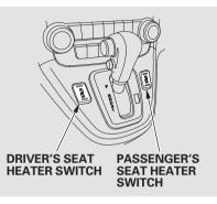
The ignition switch must be in the ON (II) position to use the heaters. Push the top of the switch, HI, to rapidly heat up the seat. After the seat reaches a comfortable temperature, select LO by pushing the bottom of the switch. This will keep the seat warm.
