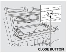
To return the screen to the upright position, press the CLOSE button on the edge of the screen panel. Do not use the folded down screen as a tray. If you put a cup, for example, on the screen, the liquid inside the cup may spill on the screen when you go over a bump. Push the AUDIO button beside the screen to show the audio display and operate the disc player.
