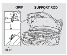
3. Holding the grip, pull the support rod out of its clip. Insert the end into the hole in the hood designated by an arrow.
