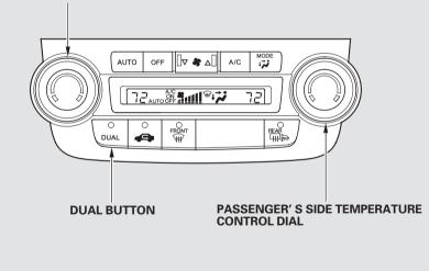
To set the driver's side temperature to a different value than the passenger's side, press the DUAL button, then turn the temperature control dial on the control panel. To set the passenger's side to a different value than the driver's side, turn the passenger's side temperature control dial. You can adjust the passenger's side without pressing the DUAL button first.
