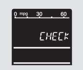
Your vehicle's onboard diagnostic system will detect a loose or missing fuel fill cap as an evaporative system leak. The first time a leak is detected a "CHECK FUEL CAP" message appears on the information display.
