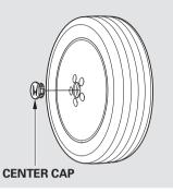
15. Remove the center cap before storing the flat tire.
