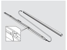
5. Place the top of the wiper blade on the end of the blade assembly, and slide the blade onto the assembly in the direction pointed to by the arrow.
