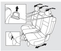
To adjust the seats forward and backward, pull up on the lever under the seat cushion. After moving the seat, make sure it is locked into position.
