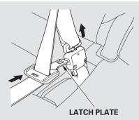
When you are folding the rear center seat-back, use the latch plate to release the center seat belt from the detachable anchor (see page 109). Allow the seat belt to retract into the holder on the ceiling and store the buckles in it.
