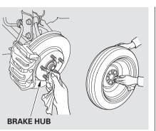
11. Before mounting the spare tire, wipe any dirt off the mounting surface of the wheel and hub with a clean cloth. Wipe the hub carefully; it may be hot from driving.
