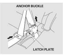
To unlatch the detachable anchor, insert the latch plate into the slot on the side of the anchor buckle. Store the detachable anchor and seat belt latch plates in the retractor housing.
