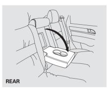
The rear seat armrest is in the center of the rear seat. Pivot it down to use it.
