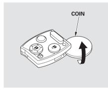
3. Inside the transmitter, separate the inner cover from the keypad by carefully prying on the edge with a coin. BATTERY
