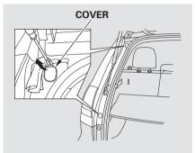
1. Open the tailgate. Place a cloth on the edge of the cover to prevent scratches. Remove the covers by carefully prying on the edge with a small flat-tip screwdriver.
