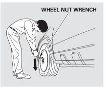
7. Loosen each wheel nut 1/2 turn with the wheel nut wrench.
