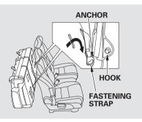
4. Pull out the fastening strap from the slit on the seat-back. Then attach the anchor on the fastening strap to the hook on the center pillar.
