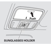
To open the sunglasses holder, push then release the raised detent. It will unlatch and swing down. To close it, push it until it latches. Make sure the holder is closed while you are driving.
