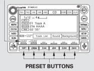
You can use the preset buttons while a disc is playing to select passages and change tracks (files in MP3 or WMA mode). Each preset button's function is shown on the bottom of the screen. You can also select an icon with the joystick. Move it to left, right, up, or down to change the highlighting and scroll through lists. Then press ENT on the top of the joystick to select the icon.
