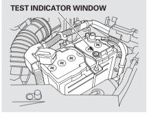
Check the condition of the battery monthly by looking at the test indicator window. The label on the battery explains the test indicator's colors.
