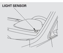
The automatic lighting feature is controlled by a sensor located on top of the dashboard. Do not cover this sensor or spill liquids on it.
