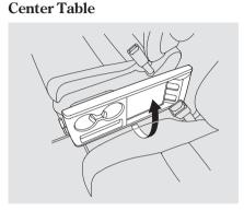
*On LX and U.S. EX models* To use the center table, pull up the outside edge of the table until it latches. To store it, pull the lever and lower the table.
