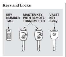
The master key fits all the locks on your vehicle. The valet key works only in the ignition and the driver's door lock. You can keep the glove box locked when you leave your vehicle and the valet key at a parking facility. You should have received a key number tag with your keys. You will need this key number if you ever have to get a lost key replaced. Use only Honda-approved key blanks.
