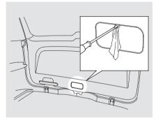
If the power door lock system cannot unlock the tailgate, unlock it manually.
