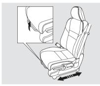
To adjust the seat forward or backward, pull up on the bar under the seat cushion's front edge. Move the seat to the desired position, and release the bar. Try to move the seat to make sure it is locked in position.
