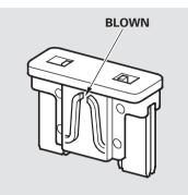
5. Look for a blown wire inside the fuse. If it is blown, replace it with one of the spare fuses of the same rating or lower.
