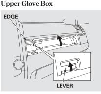
Open the upper glove box by pushing up the lever. Close it by pulling down on the edge under the lever.
