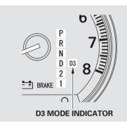
When the D3 mode is on, the transmission selects only the first three gears. Use D3 mode when towing a trailer, or to provide engine braking when going down a steep hill. D3 mode can also keep the transmission from cycling between third and fourth gears in stop-and-go driving.
