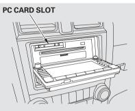
The PC card slot is behind the navigation screen. To use the PC card player, press the OPEN button beside the screen. The screen folds back, and the PC card slot appears. Insert a PC card straight into the slot. The drive will read the PC card and begin to play it.
