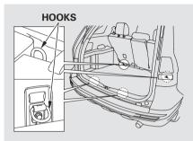
The four hooks on the floor can be used to install a net for securing items.
