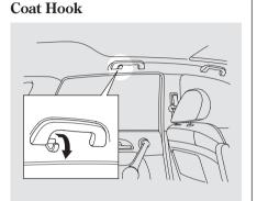
To use a coat hook, slide it out slightly, then pull it down.
