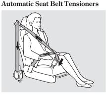
For added protection, the front seat belts are equipped with automatic seat belt tensioners. When activated, the tensioners immediately tighten the belts to help hold the driver and a front passenger in position. The tensioners can be activated during a collision in which the front airbags *do not deploy*. In this case, the airbags would not be needed, but the additional restraint could be helpful.
