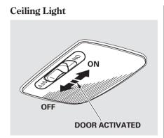
The ceiling light has a three-position switch: ON, Door Activated, and OFF. In the Door Activated (center) position, the light comes on when you:
