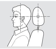
Adjust the driver's head restraint so the center of the back of your head rests against the center of the restraint.
