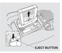
2. Push the EJECT button to remove the CD magazine. The magazine will pop up automatically.
