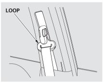
If your seat belts get dirty, use a soft brush with a mixture of mild soap and warm water to clean them. Do not use bleach, dye, or cleaning solvents. Let the belts air-dry before you use the vehicle. Dirt build-up in the loops of the seat belt anchors can cause the belts to retract slowly. Wipe the insides of the loops with a clean cloth dampened in mild soap and warm water or isopropyl alcohol.
