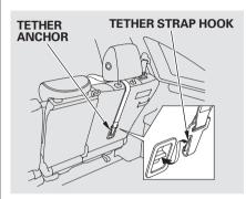
6. Route the tether strap over the seat-back and through the legs of the head restraint, then attach the tether strap hook to the anchor, making sure the tether strap is not twisted.
