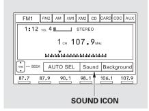
You can adjust the sound on the navigation screen. To adjust the sound, push the AUDIO button, then enter the sound grid by touching the SOUND icon on the display.
