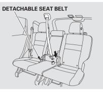
The lap/shoulder belt in the center seating position on the rear seat is equipped with a detachable seat belt that has two parts: a small latch plate and an anchor buckle.
