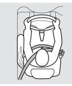
If you ever have a moderate to severe side impact, sensors will detect rapid acceleration and signal the control unit to instantly inflate either the driver's or the passenger's side airbag.
