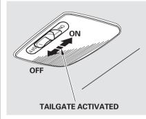
The cargo area light has a threeposition switch. In the OFF position, the light does not come on. In the center position, it comes on when you open the tailgate. In the ON position, it stays on continuously. The heating and air conditioning system in your vehicle provides a comfortable driving environment in all weather conditions.
