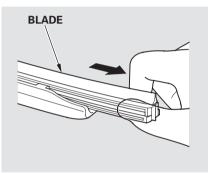
3. Remove the blade from its holder by grasping the tabbed end of the blade. Pull firmly until the tabs come out of the holder.
