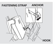
5. Pull down on the anchor to engage the upper part of the anchor securely on the hook, and make sure the seat is secure. Make sure that the folded up right rear seat does not interfere with the front passenger's seat-back. This will cause the front passenger's weight sensors and the front passenger's seat belt reminder indicator to work improperly (see page 33). Also check the passenger airbag off indicator to assure proper operation of the passenger's advanced front airbag.
