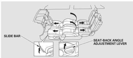
You can recline the seat-backs on the front seats so they are level with the rear seat cushions, making a large cushioned area. To do this:
