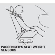
The passenger's advanced front airbag system has weight sensors under the seat. Although Honda does not encourage carrying an infant or small child in front, if the sensors detect the weight of an infant or small child (up to about 65 lbs or 29 kg), the system will automatically turn the passenger's front airbag off. Be aware that objects placed on the passenger's seat can also cause the airbag to be turned off.
