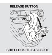
6. Remove the key from the shift lock release slot, then reinstall the cover. Make sure the notch on the cover is on the right side. Insert the key into the ignition switch, press the brake pedal, and restart the engine.
