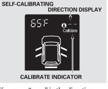
If you see "--" in the direction display when you turn the ignition switch to the ON (II) position, the compass is self-calibrating.
