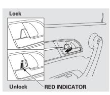
The lock tab on any passenger's door locks and unlocks that door.
