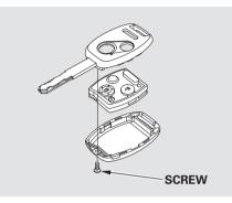
1. Remove the screw at the base of the transmitter with a small Phillips-head screwdriver.
