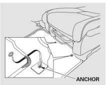
The floor mats that came with your vehicle hook over the floor mat anchors. This keeps the floor mats from sliding forward, possibly interfering with the pedals, or backwards, making the front passenger's weight sensors ineffective. If you remove a floor mat, make sure to re-anchor it when you put it back in your vehicle.
