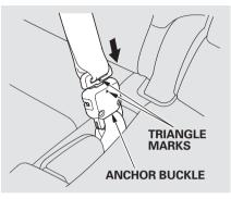
Line up the triangle marks on the small latch plate and anchor buckle when reattaching the belt and buckle.
