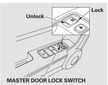
To lock all doors and the tailgate, push the top of the master door lock switch on either front door, pull the lock tab rearward on the driver's door, or use the key on the outside lock on the driver's door.
