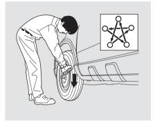
14. Tighten the wheel nuts securely in the same crisscross pattern. Have the wheel nut torque checked at the nearest automotive service facility. Tighten the wheel nuts to: 80 lbf-ft (108 N·m , 11 kgf·m)
