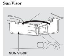
To use the sun visor, pull it down. When using the sun visor for the side window, remove the support rod from the clip, and swing it out.
