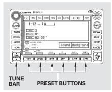
You can use the preset buttons while a disc is playing to select passages and change tracks. Each preset button function is shown on the bottom of the screen. **SKIP** – Push the  $\rightarrow$  l button (preset 6) to play the next track on the disc. Push the  $\square \blacktriangleleft$  button (preset 5) once to replay the track in play; press it twice to replay the previous track.
