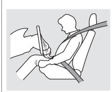
After inflating, the front airbags immediately deflate, so they won't interfere with the driver's visibility, or the ability to steer or operate other controls. The total time for inflation and deflation is one-tenth of a second, so fast that most occupants are not aware that the airbags deployed until they see them lying in their laps.
