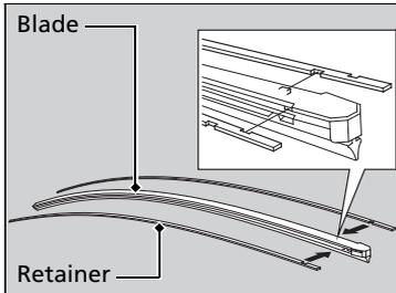
**5.** Remove the retainers from the rubber blade that has been removed, and mount to a new rubber blade.
