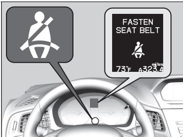
Your vehicle monitors front seat belt use. If the power mode is set to ON before the driver's seat belt is fastened, a beeper will sound and the indicator will blink. If the driver does not fasten the belt before the beeper stops, the indicator will remain on.
