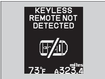
Warning buzzers may sound from inside or/ and outside the vehicle to remind you that the keyless access remote is out of the vehicle. If the buzzer continues even after the remote is put back inside, place it to be within its operational range.
