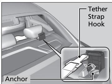
3. Open the tether anchor cover behind the head restraint.
