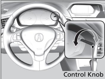
When the power mode is in ON, you can use the brightness control knob to adjust instrument panel brightness.
