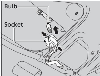
3. Remove the license plate light assembly by squeezing the tabs on both sides of the socket.
