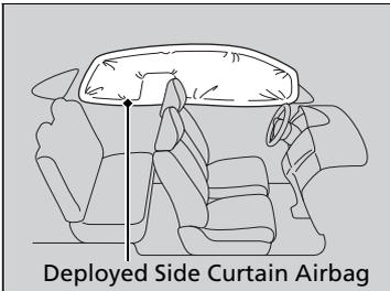
The side curtain airbag is designed to deploy in a moderate-to-severe side impact.
