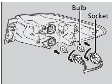
4. Turn the socket to the left and remove it.
