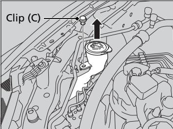
1. Remove the engine compartment cover.
