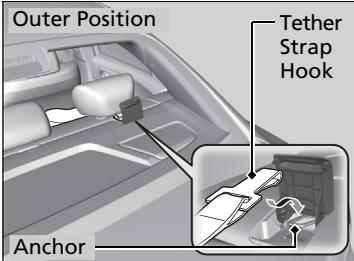
**2.** Raise the head restraint to its highest position, then route the tether strap through the head restraint legs. Make sure the strap is not twisted.
