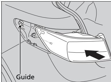
6. Reinstall the light assembly by sliding it on to the guide on the body.
