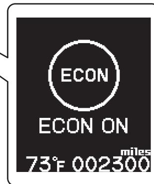
The message is displayed for a few seconds when the **ECON** mode is on.
