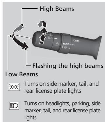
Rotating the light switch turns the lights on and off, regardless of the power mode setting.
