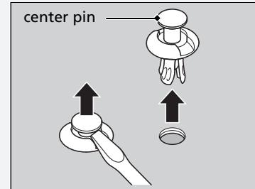
Insert the clip with the center pin raised, and push until it is flat.
