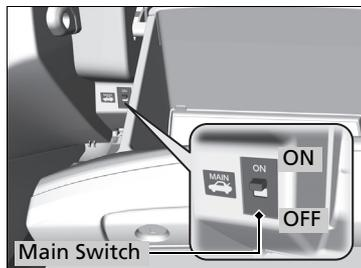
The trunk main switch disables the trunk release button on the remote transmitter and the trunk release button on the trunk lid to protect luggage in the trunk.
