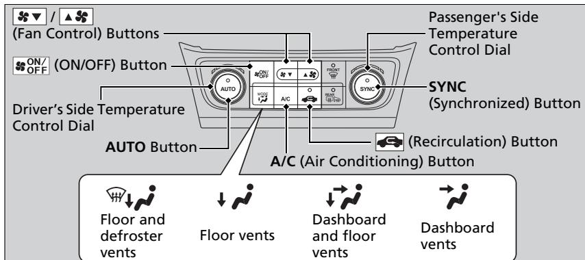
Use the system when the engine is running.
