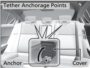
A tether anchorage point is provided behind each rear seating position. A child seat that is installed with a seat belt and comes with a tether can use the tether for additional security.
