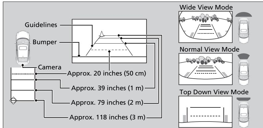
You can view three different camera angles on the rearview display. Press the selector knob to switch the angle.
