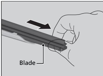
**4.** Slide the wiper blade out from its holder by pulling the tabbed end out.
