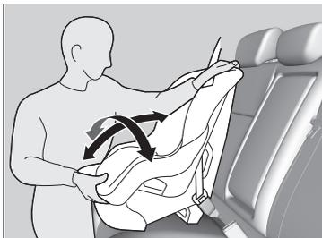
6. Make sure the child seat is firmly secured by rocking it forward and back and side to side; little movement should be felt.
