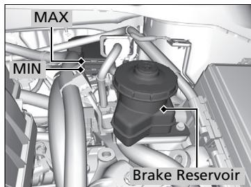
Check the fluid level several seconds after you turn the power mode to ON.
