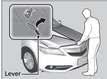
3. Slide the hood latch lever in the center of the hood to release the lock mechanism, and open the hood.
