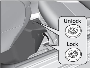
The front floor mats hook over the floor anchors, which keep the mats from sliding forward. To remove the mats for cleaning, turn the anchor knobs to the unlock position. When reinstalling the mats after cleaning, turn the knobs to the lock position.
