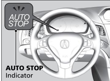
The engine then restarts once the vehicle is about to move again, and the indicator goes off.
