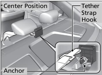
**3.** Secure the tether strap hook onto the anchor.
