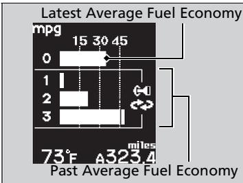
Shows the average fuel economy for the last three driving cycles (1-3), and the current driving cycle (0) in mpg or l/100 km.
