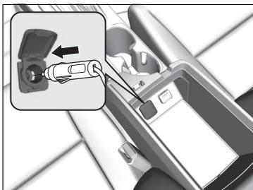
4. Plug in the compressor to the accessory power socket. Be careful not to pinch the cord in a door or window.
