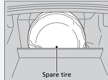
The spare tire is stored at the back of the trunk, behind the rear seat-backs.
