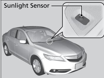
The automatic climate control system is equipped with a sunlight sensor, an interior temperature and humidity sensor. Do not cover or spill any liquid on them.
