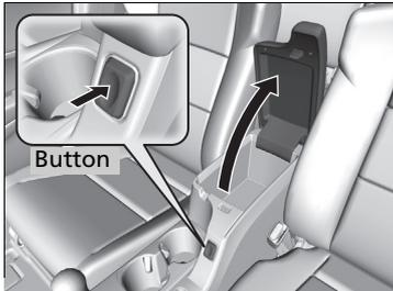
Press the button to open the console compartment.
