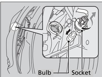
1. Turn the steering wheel all the way to the opposite side from the light being replaced.
