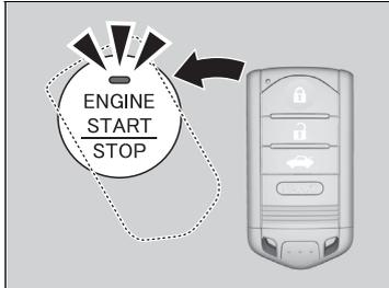
1. Touch the center of the **ENGINE START/STOP** button with the **A** logo on the keyless access remote while the indicator on the **ENGINE START/STOP** button is flashing. The buttons on the keyless access remote should be facing you.
