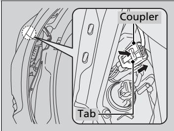
Turn the steering wheel and pull the inner fender back in the same way as when replacing the front turn signal light bulbs.
