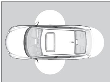
When you carry the keyless access remote, you can lock/unlock the doors and open the trunk.
