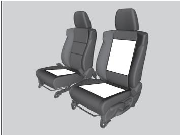
The power mode must be in ON to use the seat heaters. The **HI** setting heats the seats faster than the **LO** setting.
