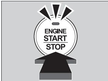
2. Depress the brake pedal and press the **ENGINE START/STOP** button within 10 seconds after the beeper sounds and the indicator stays on.
