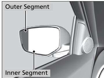
The driver side door mirror has outer and inner segments.
