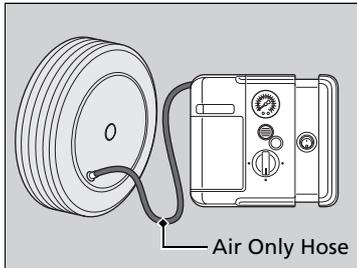
4. Recheck the air pressure using the air only hose on the compressor.
