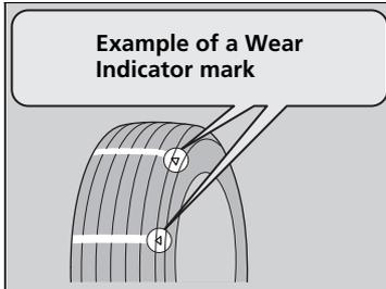
The groove where the wear indicator is located is 1/16 inch (1.6 mm) shallower than elsewhere on the tire. If the tread has worn so that the indicator is exposed, replace the tire.
