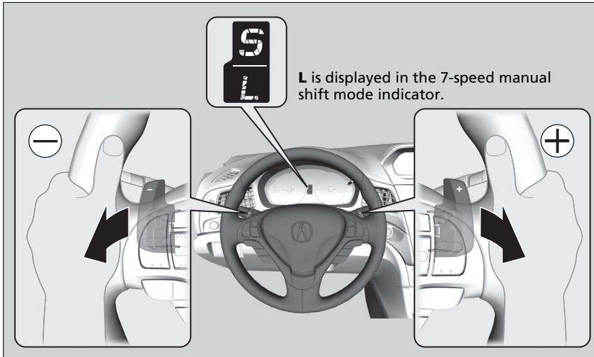
To cancel this mode, pull and hold both paddle shifters again, or move the shift lever from **[S]** to **[D]**. The **L** indicator goes off.
