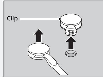
Insert the clip with the pin raised, and push until it is flat.
