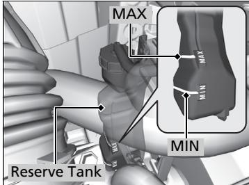
1. Check that the cooling fan is operating and stop the engine once the **ENGINE TOO HOT** message on the multi-information display goes off.
