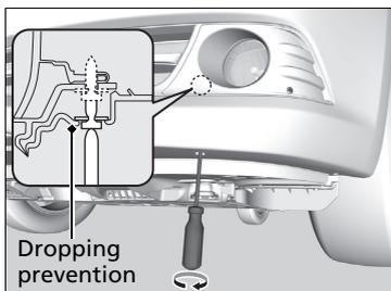
1. Remove the screw using a Phillips-head screwdriver.
