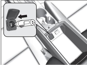
6. Plug in the kit to the accessory power socket. Be careful not to pinch the cord in a door or window.
