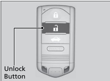
**To open:** Press the UNLOCK button twice within 10 seconds and hold it down for the second time. If the windows stop midway, repeat the procedure.
