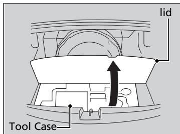
6. Pull up the trunk floor lid and take out the wheel nut wrench from the tool case.
