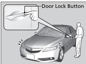
Press the door lock button on the front door.
