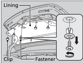
1. Remove the screw from the center of the fastener using a Phillips-head screwdriver.
