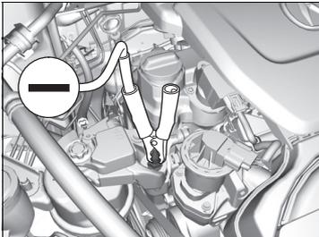
4. Connect the other end of the second jumper cable to the engine mounting bolt as shown.
