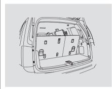
Each third row seat has a tether anchorage point behind the seat-back.
