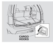
The four hooks on the side panels can be used to install a net for securing items. Each hook is designed to hold up to 50 lbs (23 kg) of weight.
