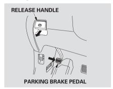
To apply the parking brake, push the pedal down with your foot. To release it, pull the release handle fully. The parking brake indicator on the instrument panel should go out when the parking brake is fully released (see page 69).
