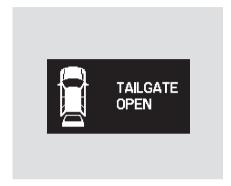
When the glass hatch, the tailgate, or both glass hatch and tailgate are not tightly closed, the "HATCH OPEN," "TAILGATE OPEN," or "HATCH & TAILGATE OPEN" message will come on.
