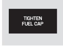
Your vehicle's on board diagnostic system will detect a loose or missing fuel fill cap as an evaporative system leak. The first time a leak is detected a "TIGHTEN FUEL CAP" message appears on the multi-information display. Turn the engine off, and confirm the fuel fill cap is installed. If it is, loosen it, then retighten it until it clicks at least once. The message should go off after several days of
