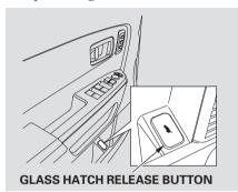
You can also open the glass hatch by pressing the glass hatch release button on the driver's door or on the remote transmitter.
