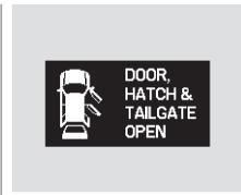
When the glass hatch, tailgate, and one or more doors are not tightly closed, the "DOOR, HATCH & TAILGATE OPEN" message will come on.
