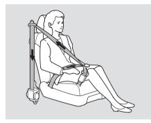
For added protection, the front seat belts are equipped with automatic seat belt tensioners. When activated, the tensioners immediately tighten the belts to help hold the driver and a front passenger in position. The tensioners are designed to activate in any collision severe enough to cause the front airbags to deploy, or if a sensor detects your vehicle is about to roll over (see page 32).
