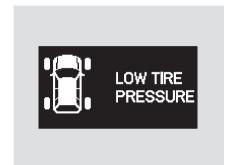
If any of the tires has low pressure, the tire pressure monitor also shows the above message to warn you about the low tire pressure when you select the display by pressing the INFO button several times. Following this display, press the SEL/RESET button to see each tire pressure. When you continue driving after installing the spare tire, you will also see this message on the multi-information display.
