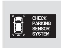
If the system develops a problem, you will see a "CHECK PARKING SENSOR SYSTEM" message on the multi-information display, and a beeper sounds continuously. Very often, a sensor covered with mud, ice, snow, etc. is the cause of this message. Check the sensors first. If the message stays on or the beeper does not stop, have the system checked by your dealer.
