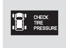
Each tire has its own pressure sensor. If the air pressure of a tire becomes significantly low, the sensor in that tire immediately sends a signal that causes the low tire pressure/TPMS indicator in the instrument panel to come on. If this happens, you will see which tire is losing pressure on the multi-information display along with a "CHECK TIRE PRESSURE" message.
