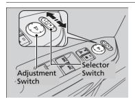
You can adjust the door mirrors when the ignition switch is in ON  $\boxed{II}$ .
