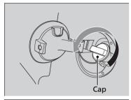
**4.** Remove the fuel fill cap slowly. If you hear a release of air, wait until this stops, then turn the knob slowly to open the fuel fill cap.
