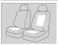
The ignition switch must be in ON  $\overline{\rm II}$  to use the seat heaters. The  ${\rm HI}$  setting heats the seats faster than the  ${\rm LO}$  setting.
