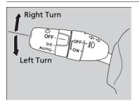
The turn signals can be used when the ignition switch is in ON  $\boxed{II}$ .
