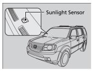
The automatic climate control system is equipped with a sunlight sensor, an interior temperature and humidity sensor. Do not cover or spill any liquid on them.
