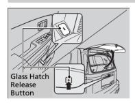
To open the glass hatch, press the glass hatch release button in the driver's door or press the button on the tailgate for about one second.
