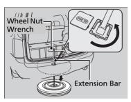
5. Put the extension bar with the wheel nut wrench on the hoist shaft. Turn the wrench to the left to lower the spare tire to the ground.
