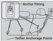
A tether anchorage point is provided behind each second and third row seating position. A child seat that is installed with a seat belt and comes with a tether can use the tether for additional security.
