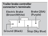
Have a qualified mechanic install your trailer brake controller following the trailer brake controller manufacturer's instructions. Failure to properly install the trailer brake controller may increase the distance it takes for you to stop your vehicle when towing a trailer.
