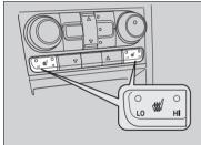
The appropriate indicator will be on while the seat heater is on. Each time you press the switch, the mode changes to **HI**, **LO** and OFF.
