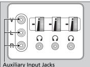
The system also allows for auxiliary inputs from standard video games. The jacks are on the back of the center console compartment.
