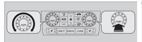
You can set the temperature synchronously for the driver side, the passenger side, and the rear passenger compartment in synchronized mode.
