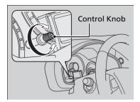
When the ignition switch is in ON  $\overline{II}$ , you can use the brightness control knob to adjust instrument panel brightness.
