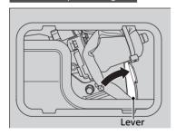
**2.** To open the tailgate, push the tailgate while sliding the lever to the right.
