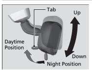
Flip the tab to switch the position.
