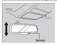
When driving after dark, the automatic dimming rearview mirror always reduces the glare from headlights behind you.
