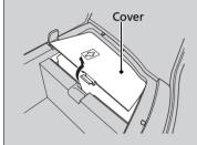
**2.** Remove the cover and take the jack, stay, wheel nut wrench, and extension bar out of the tool case.
