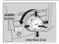
Press the **AUDIO** button, and move  $\cite{O}$  to select **AUDIO MENU**. Rotate  $\cite{O}$  to select **Sound Setup**, then press  $\cite{O}$ . Rotate  $\cite{O}$  to scroll through the following choices:
