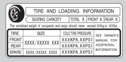
This figure includes the total weight of all occupants, cargo, and accessories, and the tongue load if you are towing a trailer. Steps for Determining Correct Load Limit -
