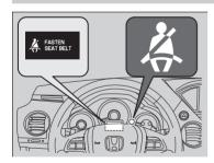
Your vehicle monitors front seat belt use. If the ignition switch is turned to ON II before the driver's seat belt is fastened, a beeper will sound and the indicator will blink. If the driver does not fasten the belt before the beeper stops, the indicator will remain on.
