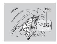
Remove the clips using a flat-tip screwdriver, and pull down the under cover. Fog Light Bulbs\*
