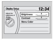
If you select **Brightness** or **Contrast**, adjust the setting by rotating  $^{\circ}$  and pressing  $^{\circ}$ .
