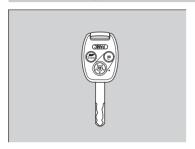
Use the keys to start and stop the engine, and to lock and unlock all the doors and tailgate. You can also use the remote transmitter to lock and unlock the doors and tailgate.
