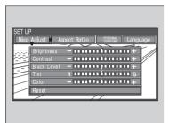
Press the **SETUP** button while the DVD is playing to see the available options. Use the ◀ and ▶ buttons to highlight the option and then press **ENT**.
