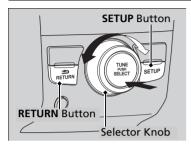
Press the **SETUP** button, and rotate to select **Sound Settings**, then press . Rotate to scroll through the following choices:
