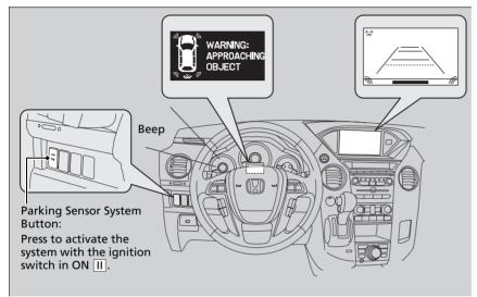
The indicator in the button comes on and the beeper sounds when the system is on.
