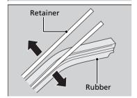
**4.** Remove the retainers from wiper blade and mount it to a new rubber blade.
