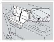
Pull the lever and lift the lid to open the compartment.
