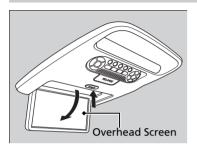
Press the **OPEN** button and pull down the screen to the first or second detent until it latches.
