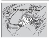
Check the battery condition monthly. Look at the test indicator window and check the terminals for corrosion.
