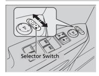
If activated, either side door mirror automatically tilts downward when you put the shift lever in  $\boxed{R}$ ; this improves close-in visibility on the selected side of the vehicle when reversing. The mirror automatically returns to its original position when you shift out of  $\boxed{R}$ .
