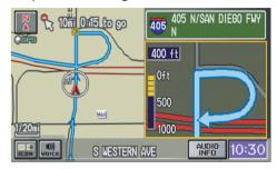
On the map screen, the location of the maneuver is marked with a small yellow square. The guidance window is simply an enlargement of the area indicated by the yellow square. After you complete the maneuver, the display returns to a full map screen when the single-screen mode is set, or to a map and direction list screen when the split-screen mode is set.
