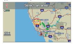
Use the joystick to move the crosshairs to the area of the state close to your intended destination. If desired, use the **ZOOM** buttons to change the map scale. When you have the crosshairs in the desired area, push in on the joystick. The address of the location you have selected will appear at the top of the screen.
