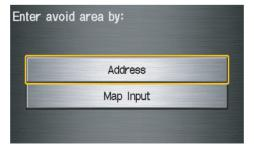
Either select **Address** or **Map Input** on the Enter avoid area by screen. Each choice provides a slightly different way to locate the approximate map display for drawing the area you wish to avoid. After selecting the choice, a map screen will be displayed.
