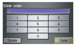
Enter the four-digit security code, then select **Done**. If you make a mistake, the system will display "incorrect PIN." Reenter your 4-digit security code. If you have entered it correctly, the display changes to the **Disclaimer** screen.
