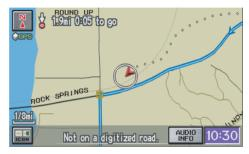
The map screen starts displaying a series of dots (breadcrumbs) to show the path you have taken if **Off-road Tracking** on the **Setup** screen (second) is set to **On** (see page 92).
