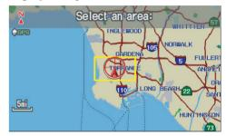
The red arrow indicates your vehicle position. Find your desired destination by moving the joystick left, right, up, or down. The map and crosshairs will move in the same direction.
